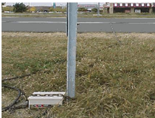
Fig 2.6: Pneumatic tube technology is used to collect vehicle classification data (Contact System)
