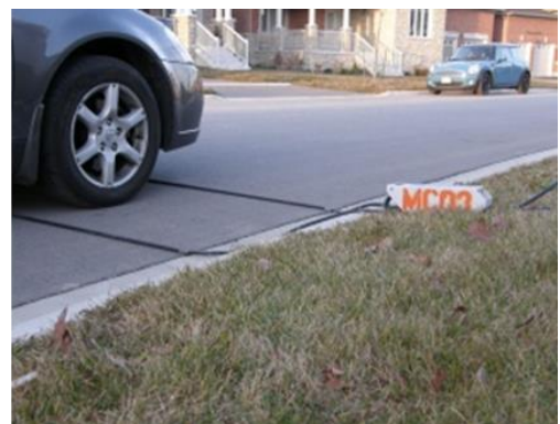
Fig 2.6: Pneumatic tube technology is used to collect vehicle classification data (Contact System)
