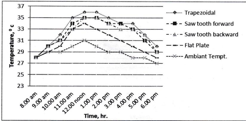
Fig. 16. Temperature distribution of Air Channel temperature on 30/04/2012.
