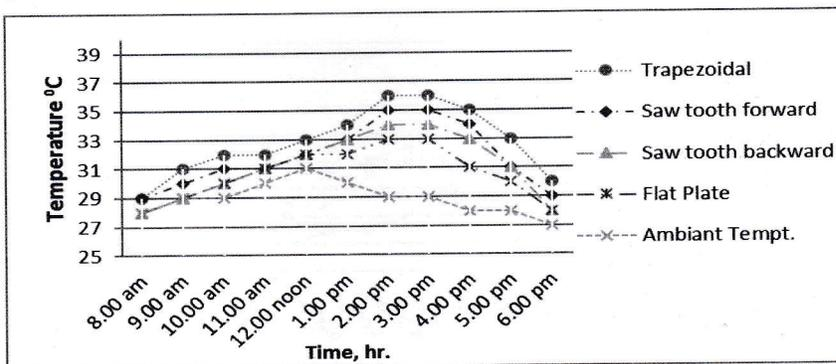
Fig. 20 Temperature distribution of Ribbed surface temperature on 15/05/2012.
