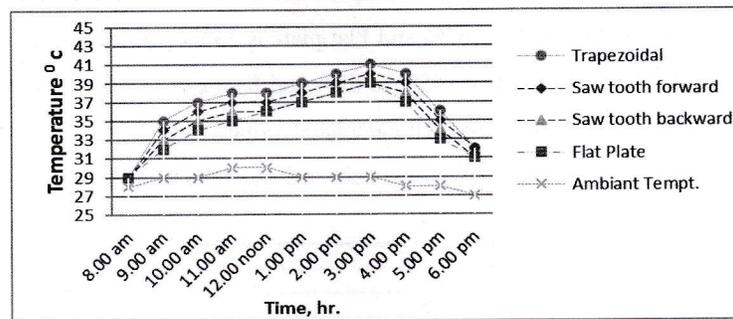
Fig. 8. Temperature distribution of PV panel temperature on 30/05/2012.
