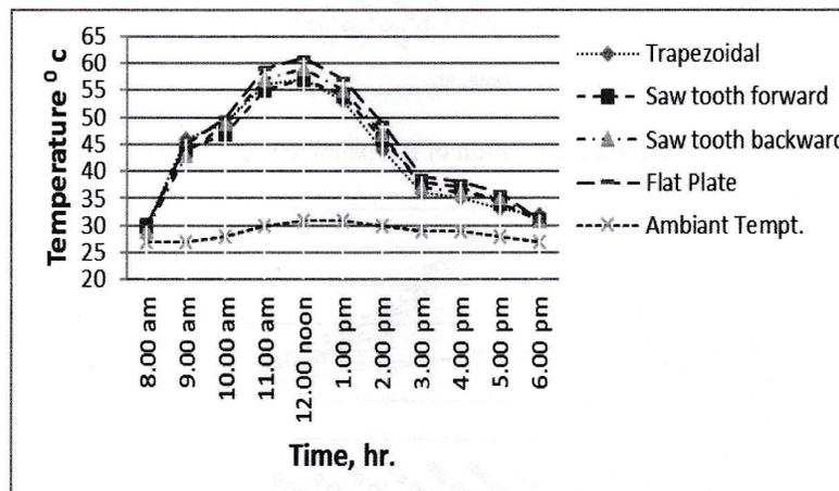
Fig. 6. Temperature distribution of PV panel temperature on 15/03/2012.
