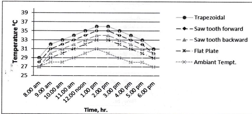
Fig. 18. Temperature distribution of Ribbed surface temperature on 15/03/2012.
