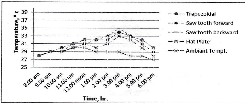
Fig. 17. Temperature distribution of Air Channel temperature on 30/05/2012.
