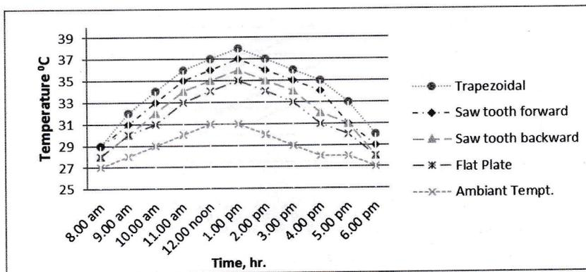
Fig. 19. Temperature distribution of Ribbed surface temperature on 15/04/2012.
