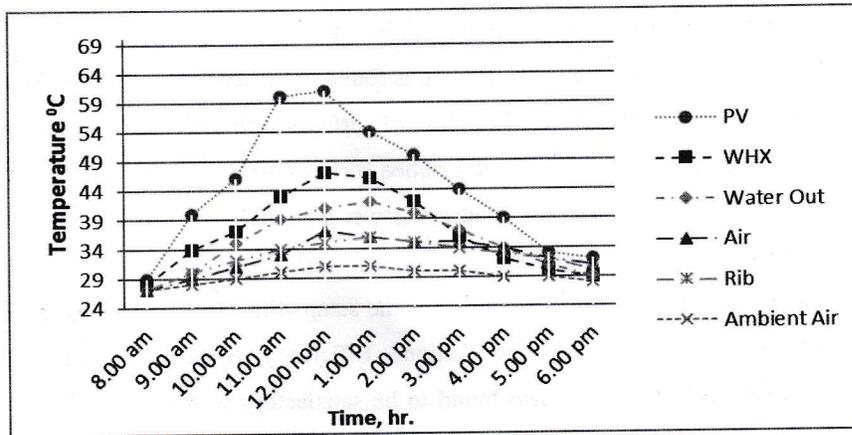
22. Temperature distribution in Saw tooth backward ribbed setup in April, 2012.
