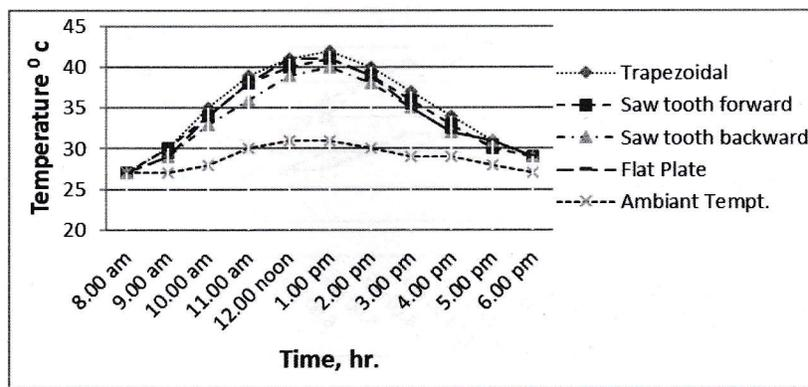
Fig. 12. Temperature distribution of water outlet temperature on 15/03/2012.
