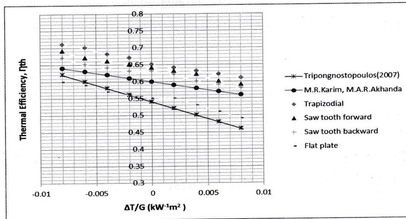
Fig. 23. Comparison of Thermal efficiencies of all four systems.
