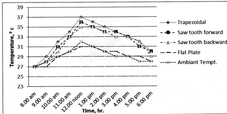
Fig. 15. Temperature distribution of Air Channel temperature on 30/03/2012.
