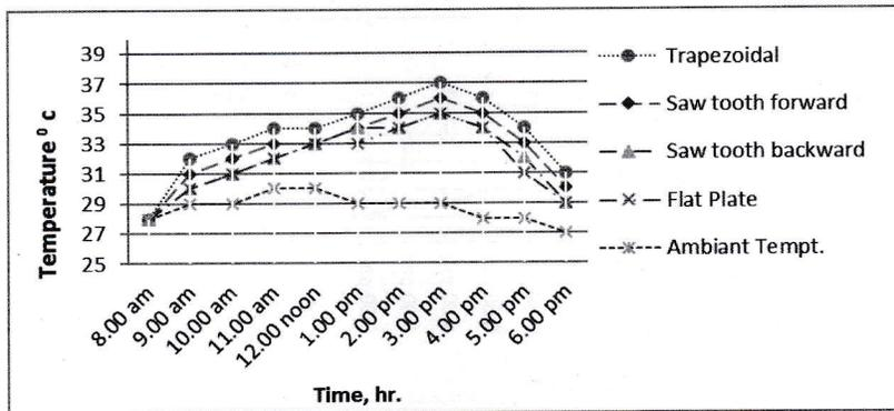
Fig. 14. Temperature distribution of water outlet temperature on 30/05/2012.
