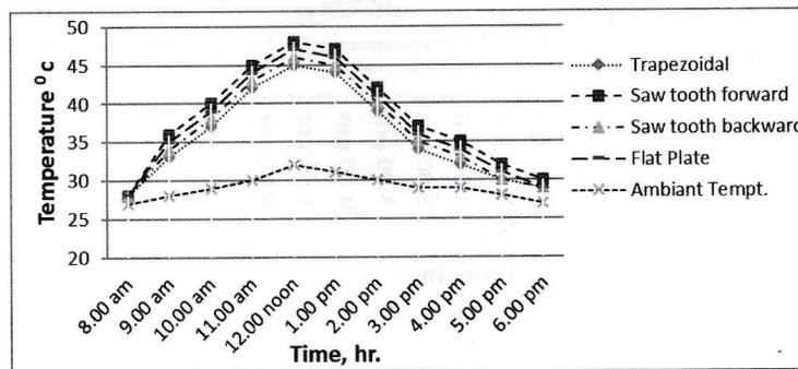
Fig. 9. Temperature distribution of water heat exchanger temperature on 30/03/2012.
