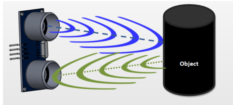
Fig.2.9.3: HC-SR04 Ultrasonic Sensor – Working.
