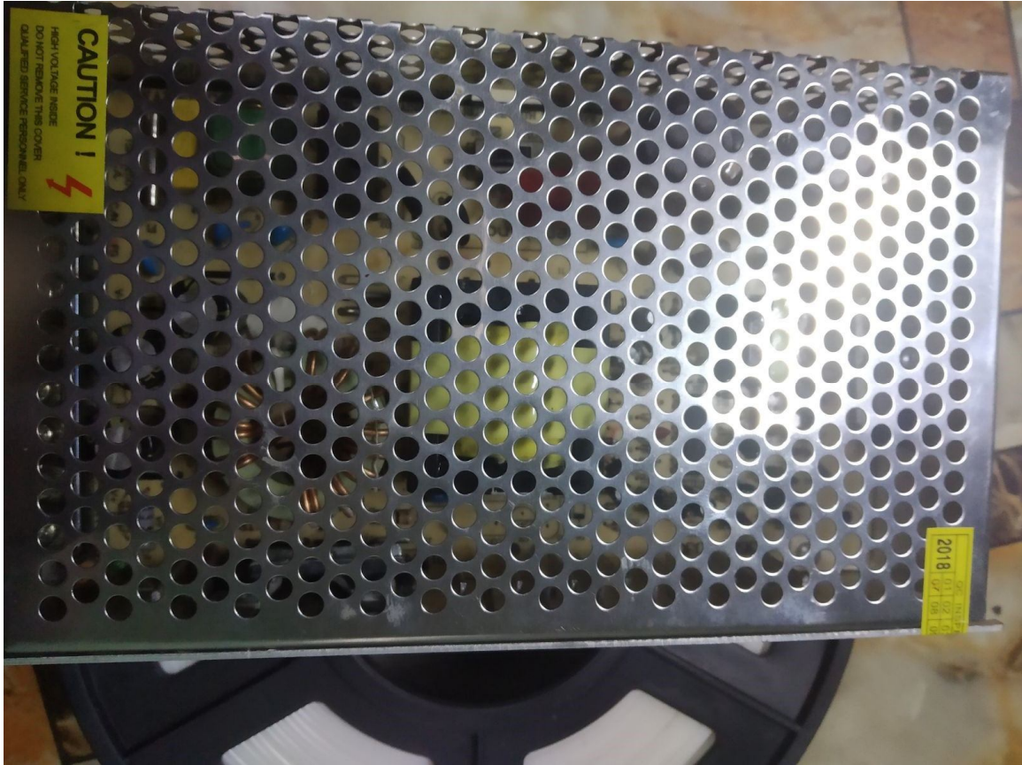
Figure(3.19): power supply 12 Volt 20 amp
