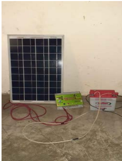
Figure 4.4: Connection with Solar Panel, Charging Controller and Battery
