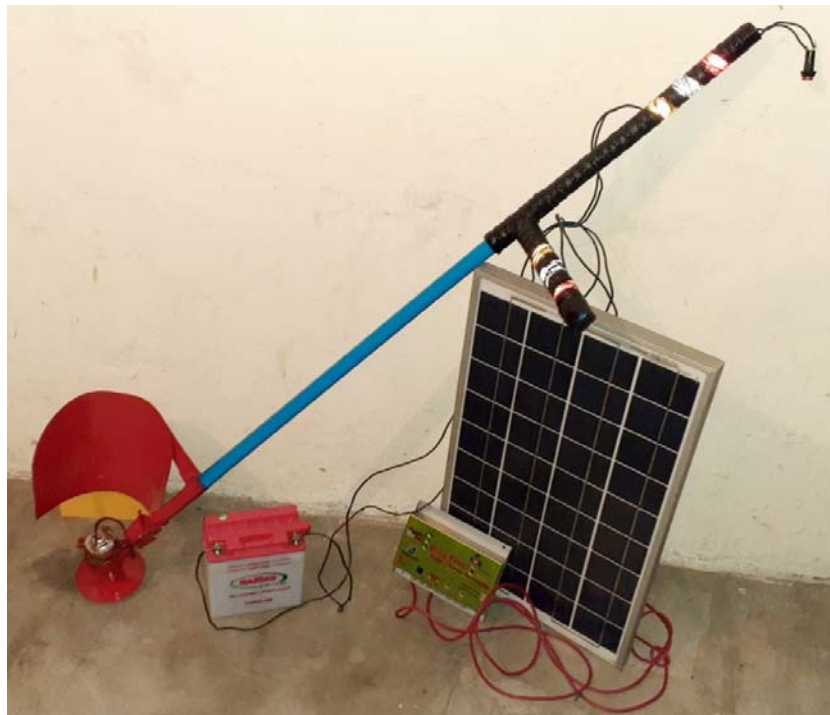
Figure 4.8: Schematic diagram of solar based paddy harvesting machine
