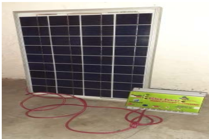
Figure 4.3: Connection with Solar Panel and Charging Controller
