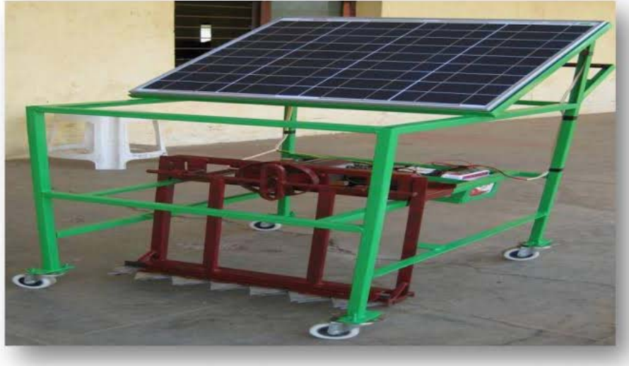
Figure 2.3:Solar Grass Cutter with Linear Blades by Using Scotch Yoke Mechanism
