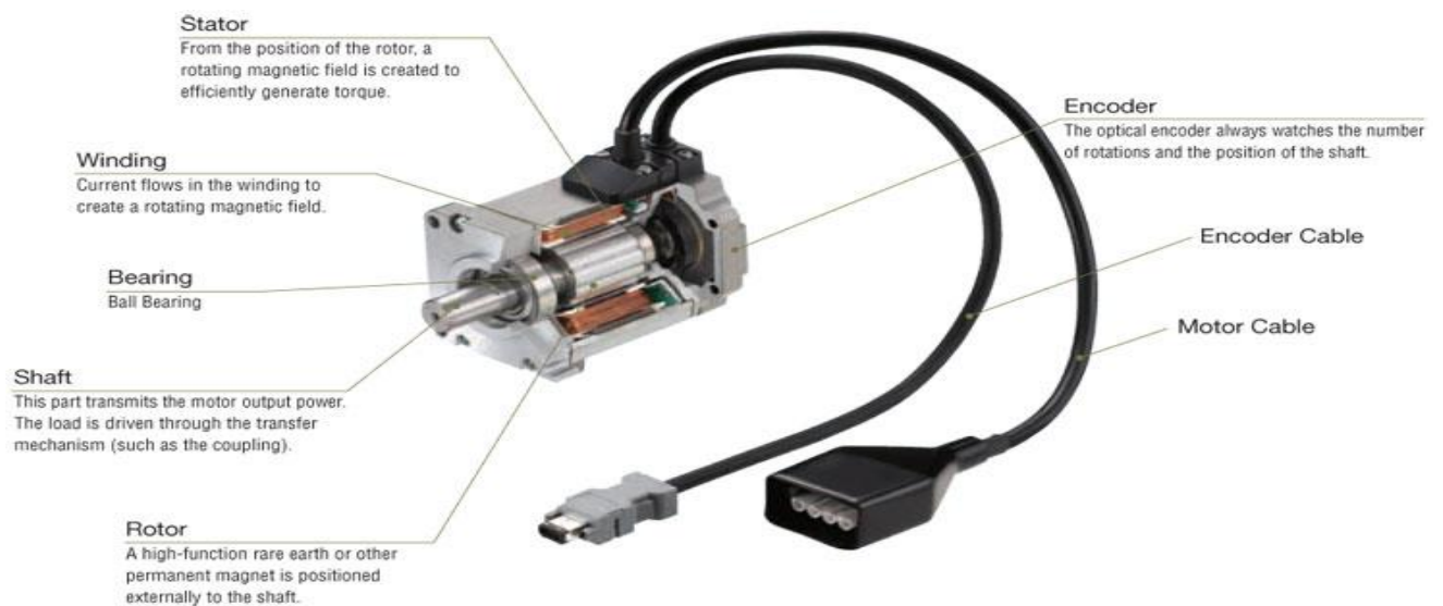
Fig 3.8.3 : Servo motor all parts
