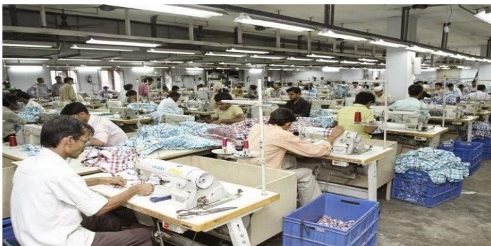
Figure-2. Straight line operator facing opposite direction
