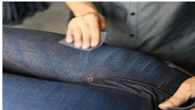
Fig: Marked Scraping Area
