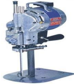
Fig: Straight Knife cutting machine
