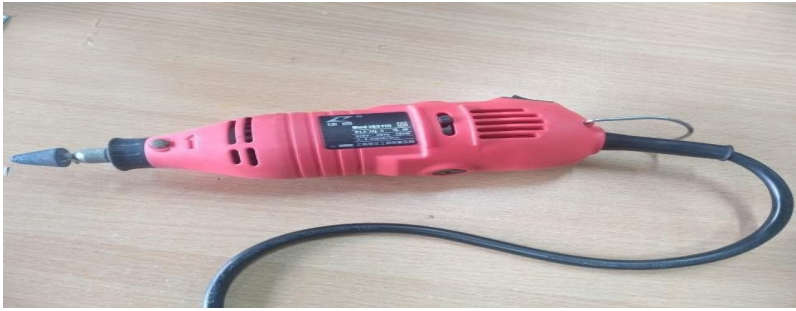
Figure: Grinding Machine
