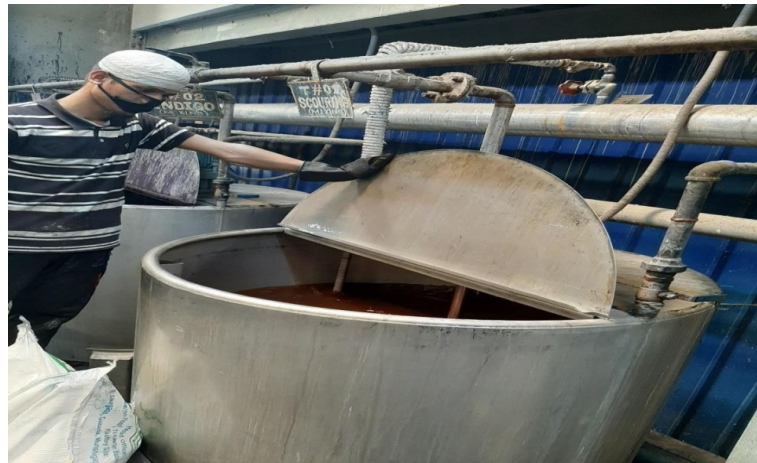
Figure: Caustic Soda Mixing Box
