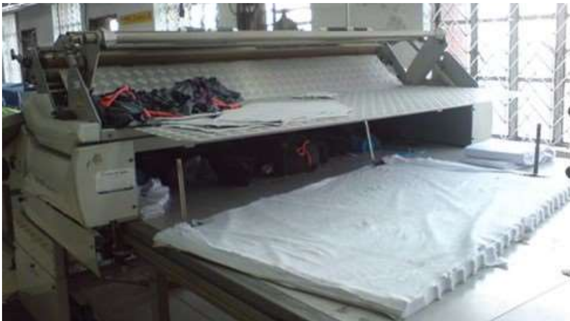
Figure: Automatic spreading Machine with fabric control devices
