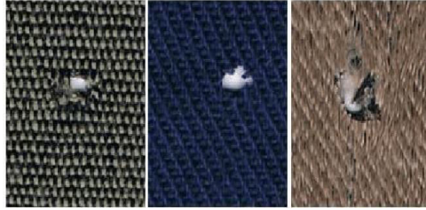
Fig: Holes in fabric
