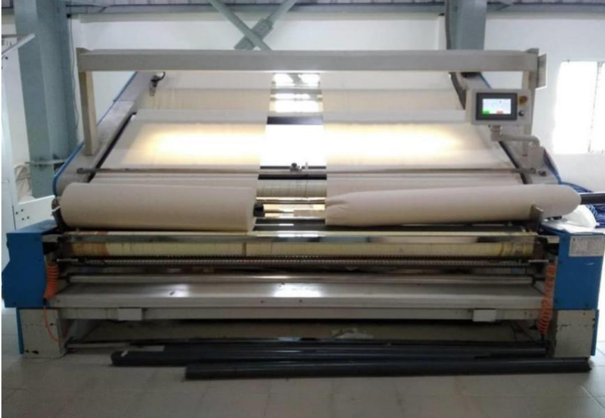
Picture: 3.2.19.1 fabric inspection
