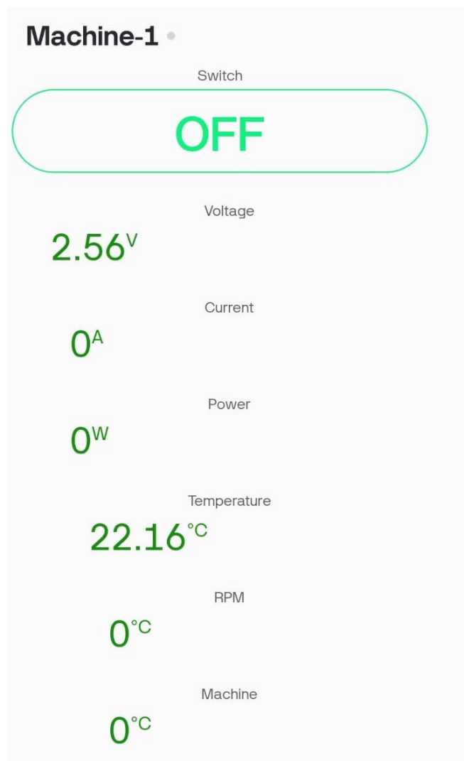
Figure 4.6: Machine 1, Motor Status Control and Monitoring
