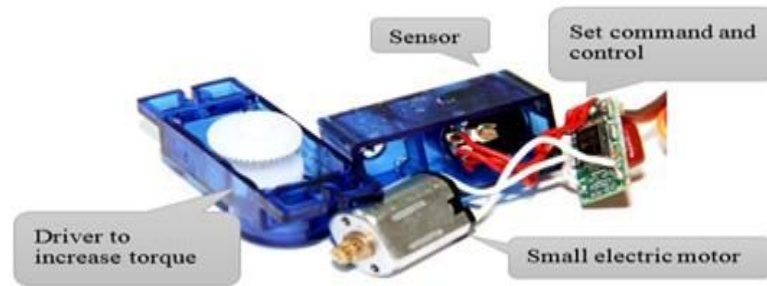
Figure 3.6: Physical Construction of Servo SG-90
