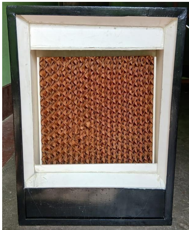
Fig: 4.7: Evaporative Water Recycling using Honey Comb (Paper Made) Pad.
