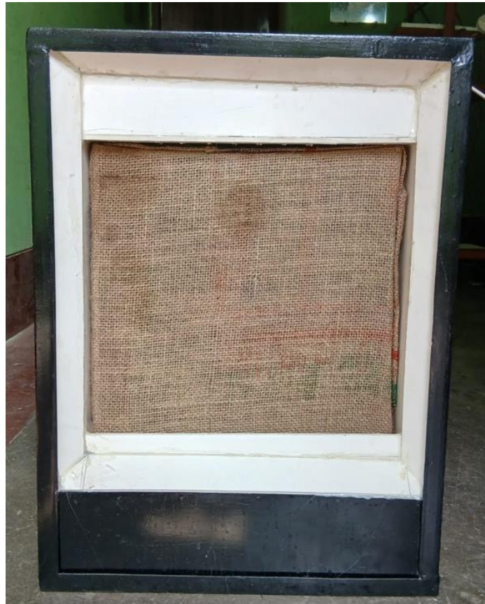
Fig: 4.6: Evaporative Water Recycling using Jute Pad.
