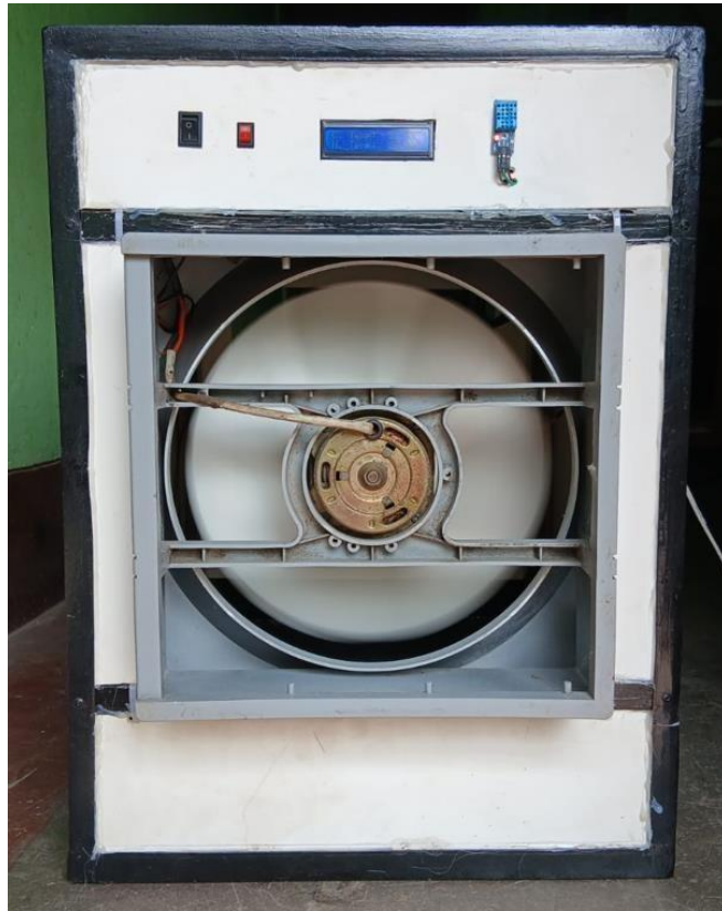
Fig: 4.4: Front View of Blower Fan.
