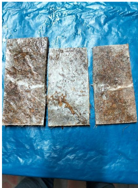
Figure: 5.7 Bending Test Specimens After Testing
