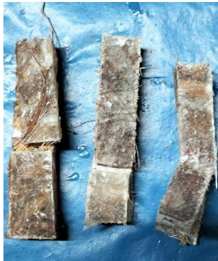
Figure: 5.4 Impact test specimens showing fracture patterns after testing
