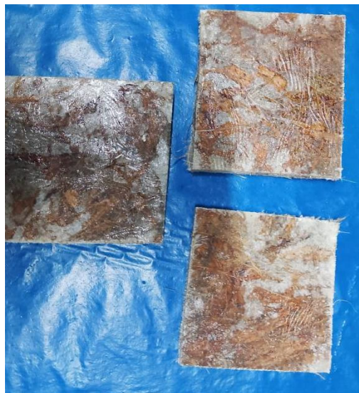
Figure: 5.1 Hardness test specimens after testing
