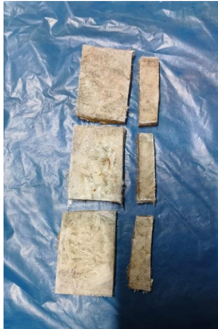
Figure: 5.4 Impact test specimens showing fracture patterns after testing
