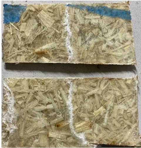
Figure: 5.7 Bending Test Specimens After Testing
