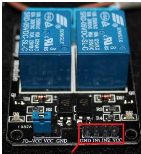
Figure 3.11: Main Voltage Connection
