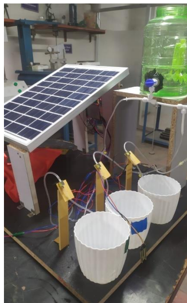
Fig 3.1: Experimental Diagram of proposed System
