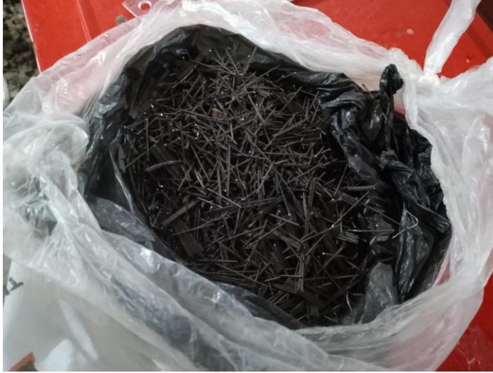
Figure 3-3. Steel Fiber 25 mm
