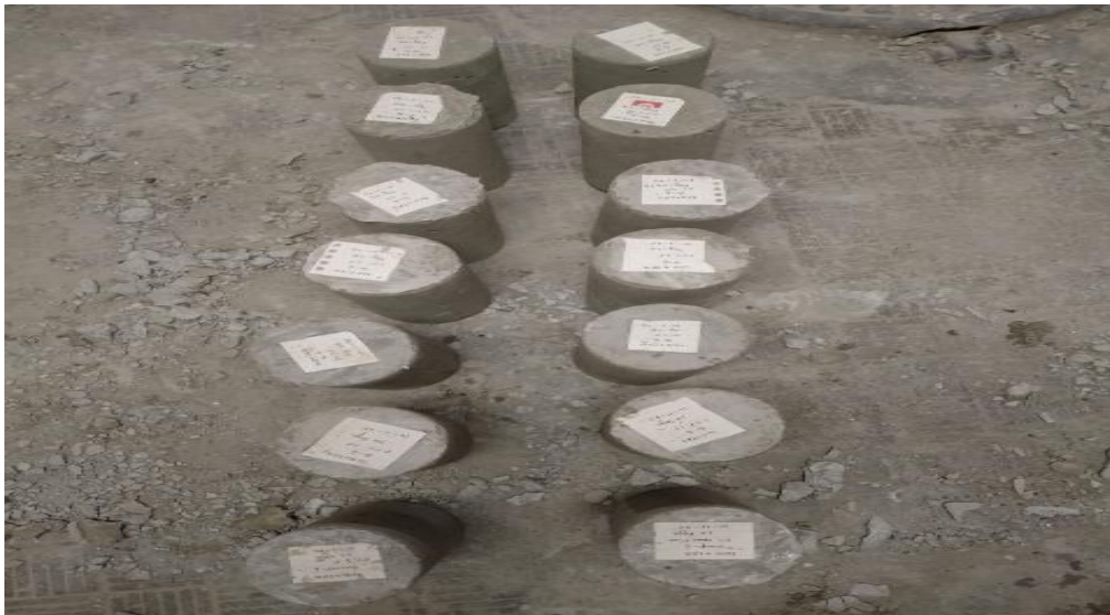
Figure: 3-18. After curing of casting cylinder
