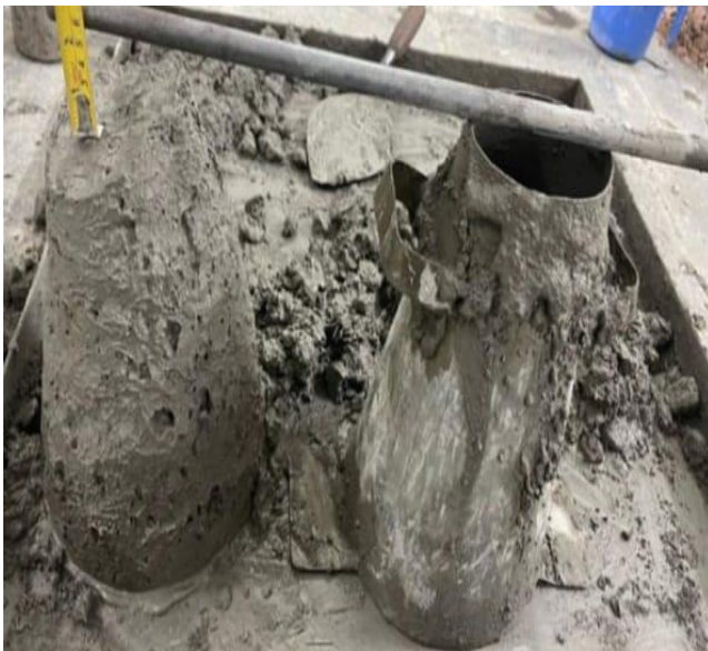
Figure: 3-14. Slump Test
