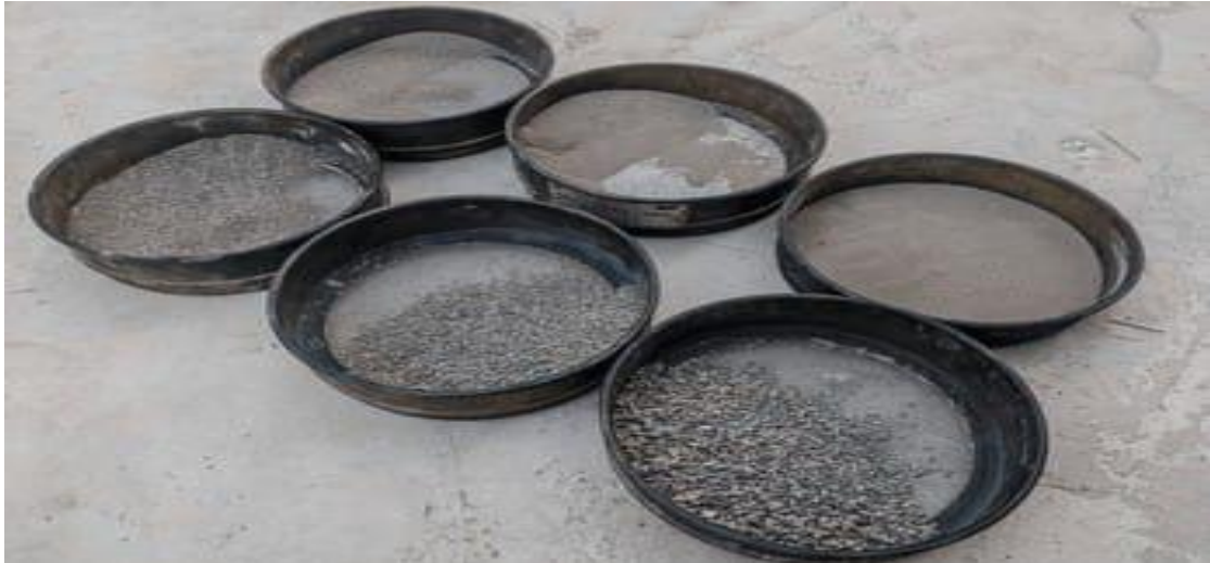
Figure 3-7. For coarse aggregate Standard Sieve.
