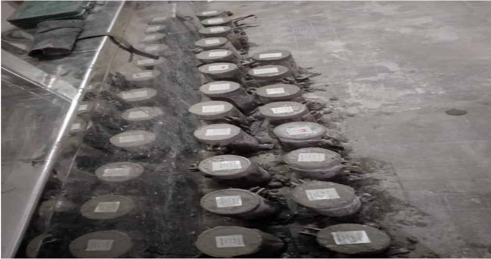
Figure: 3-16. After casting cylinder
