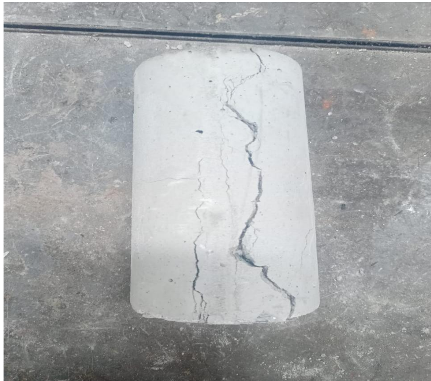
Figure 3-25. Failure of Cylinder Specimen
