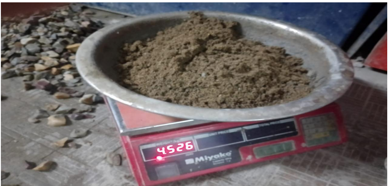
Figure 3-8. Sylhet Sand (FM 2.5 mm)
