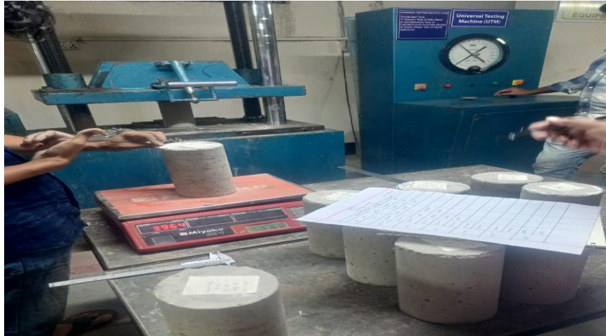
Figure 3-20. Compressive Strength Testing Machine
