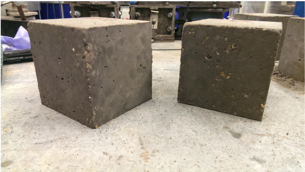
Figure 3.1: Picture of Concrete blocks using Duconmix-WR 700 made by BWDB
