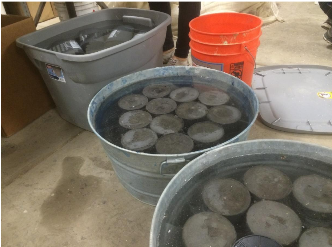
Figure 3.9: Curing of Concrete
