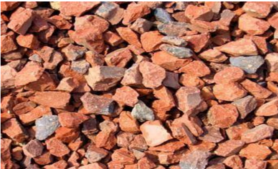
Figure 3.3: Picture of Brick Aggregate
