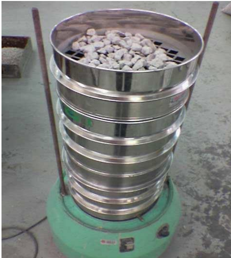
Figure 3.8 Aggregate Sieve Analysis
