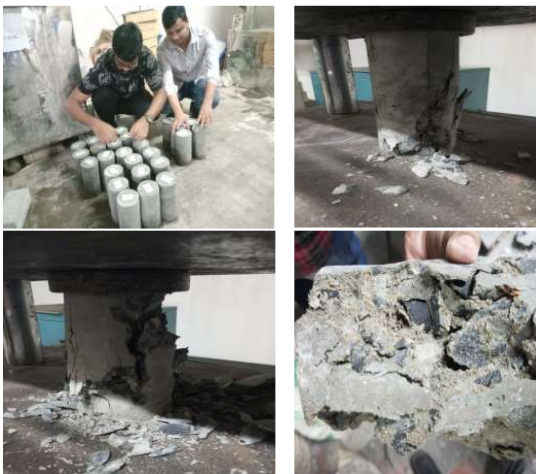
Figure: 3.10 Compressive Strength Testing
