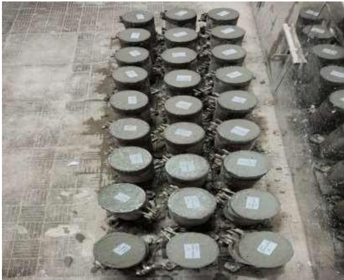
Figure 6: Mold of Cylinder
