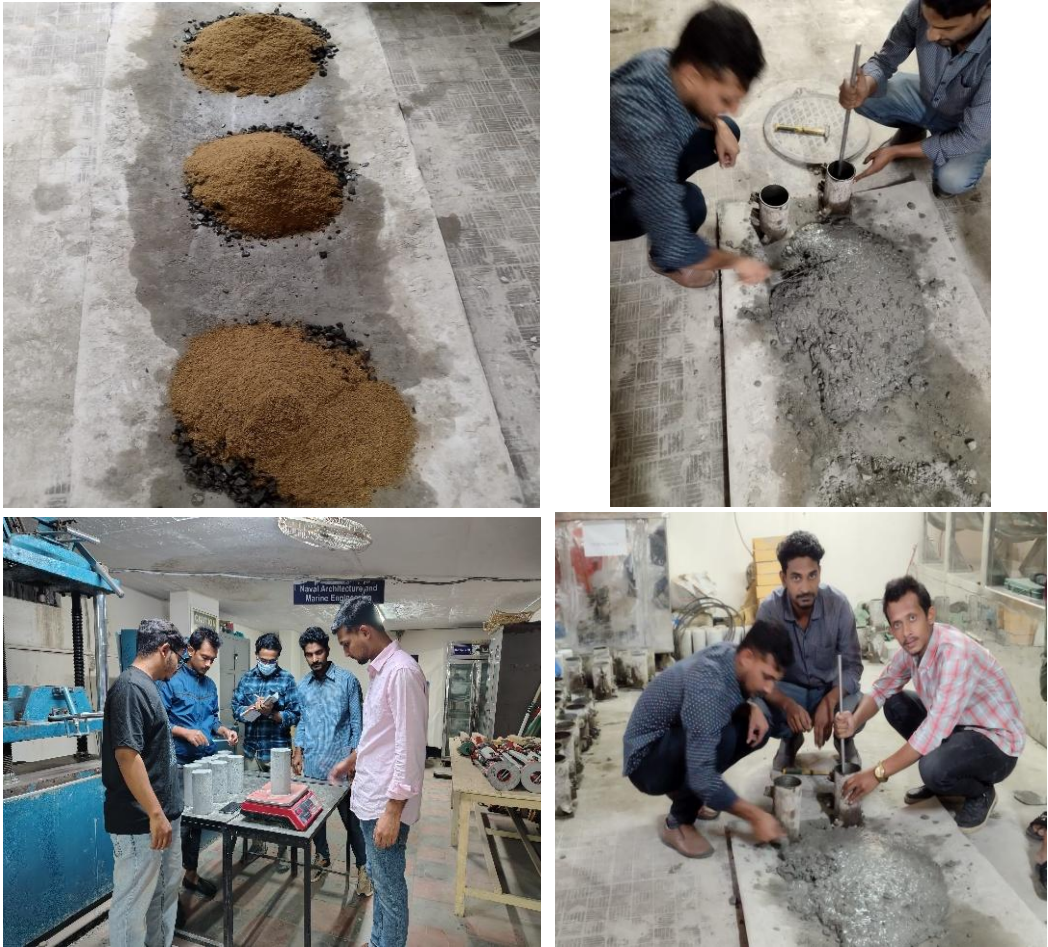
Figure 5: Concrete mixing and molding
