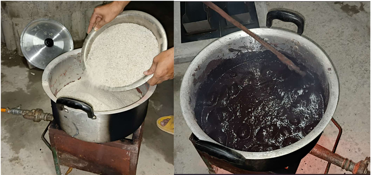
Figure 11: Pouring waste plastic into containers and melting the plastic.
