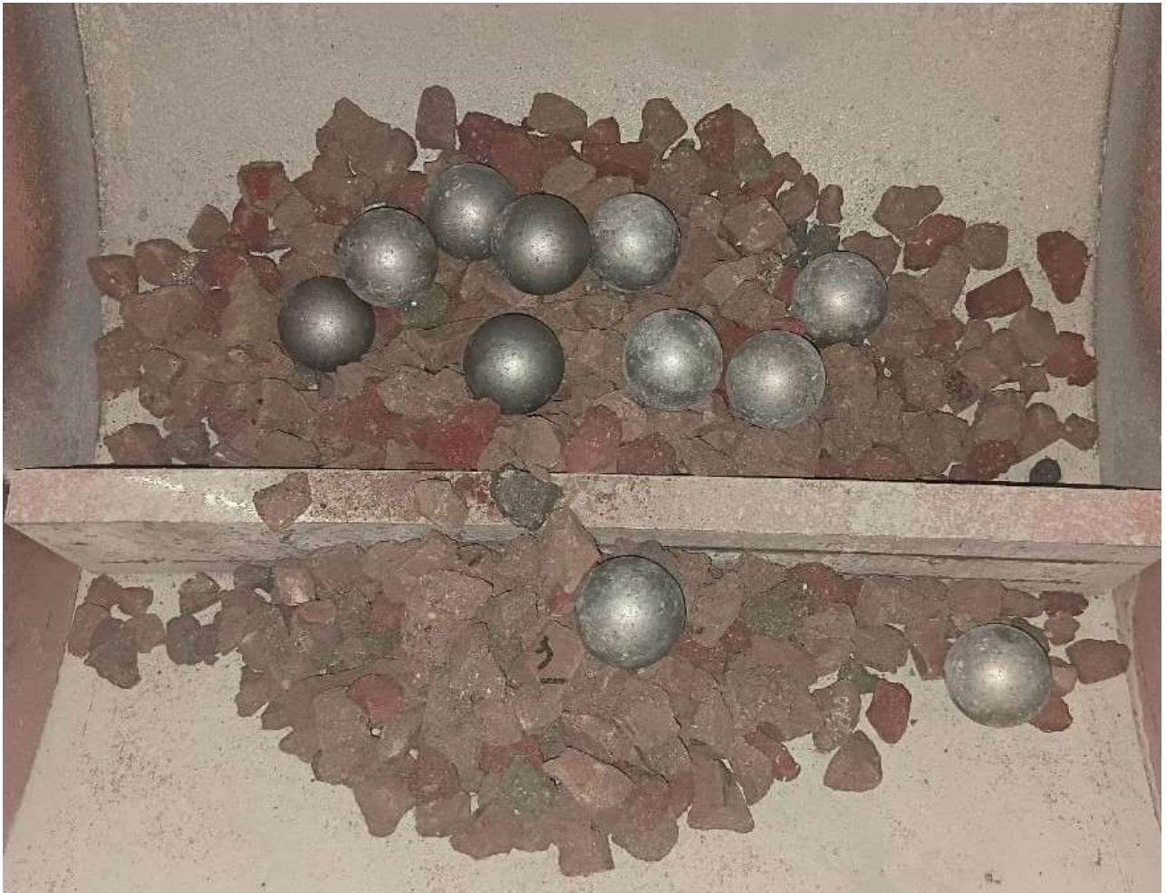
Figure 22: Steel balls and materials inside the Los Angeles machine.
