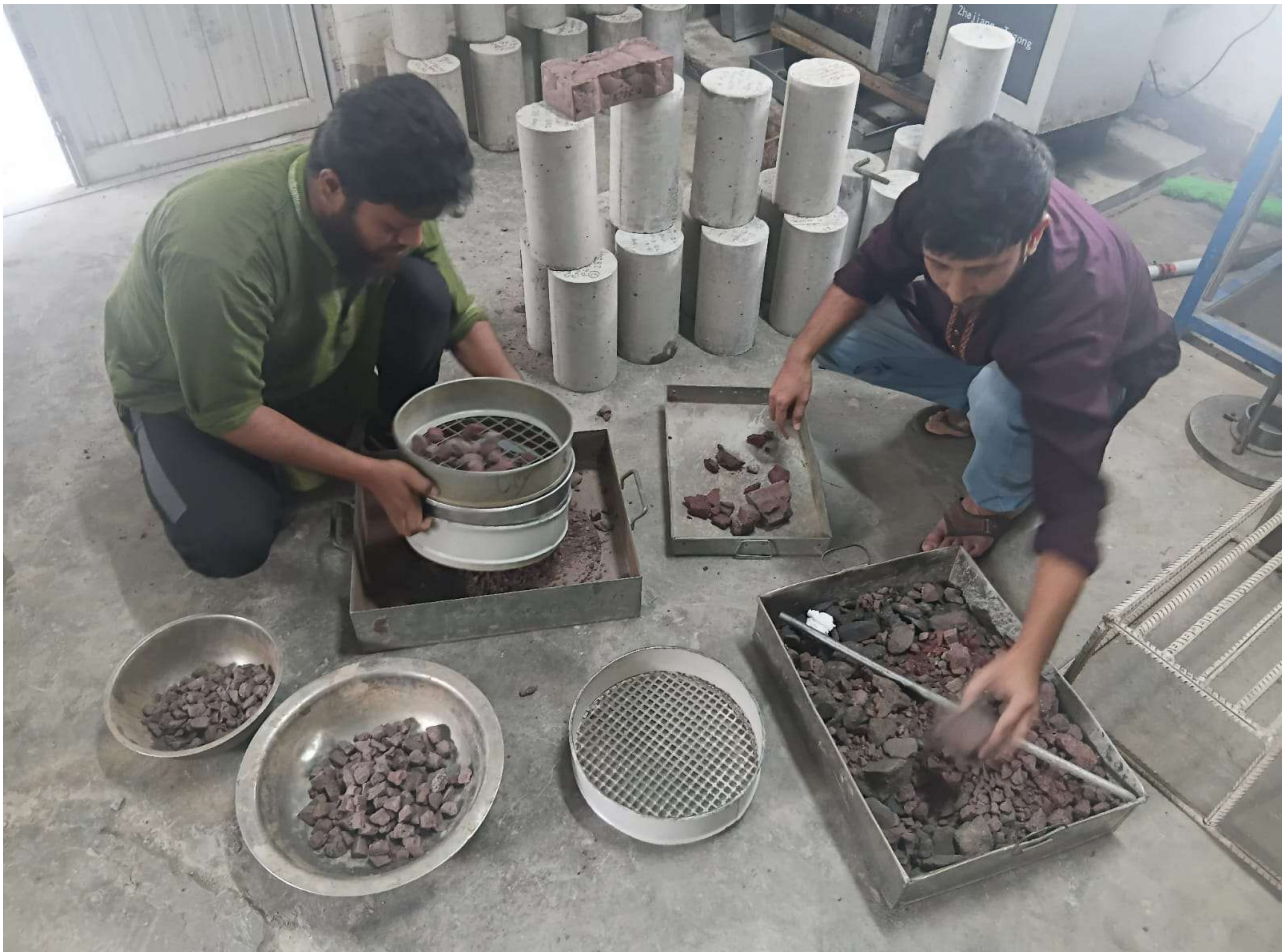
Figure 20: The khoa is being sieved for the Abrasion testing.
