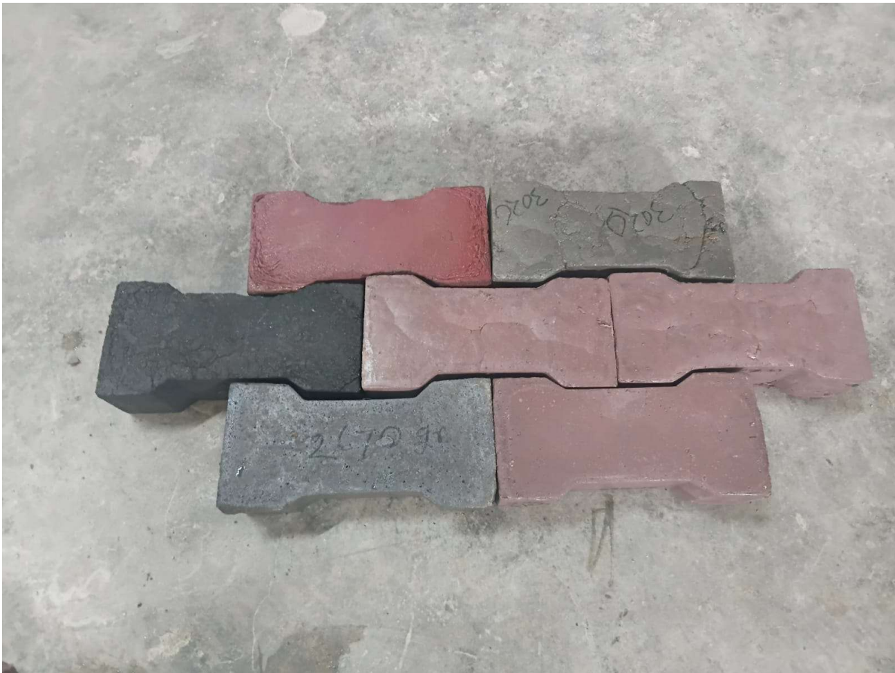
Figure 16: Open Brick from mold after Drying
