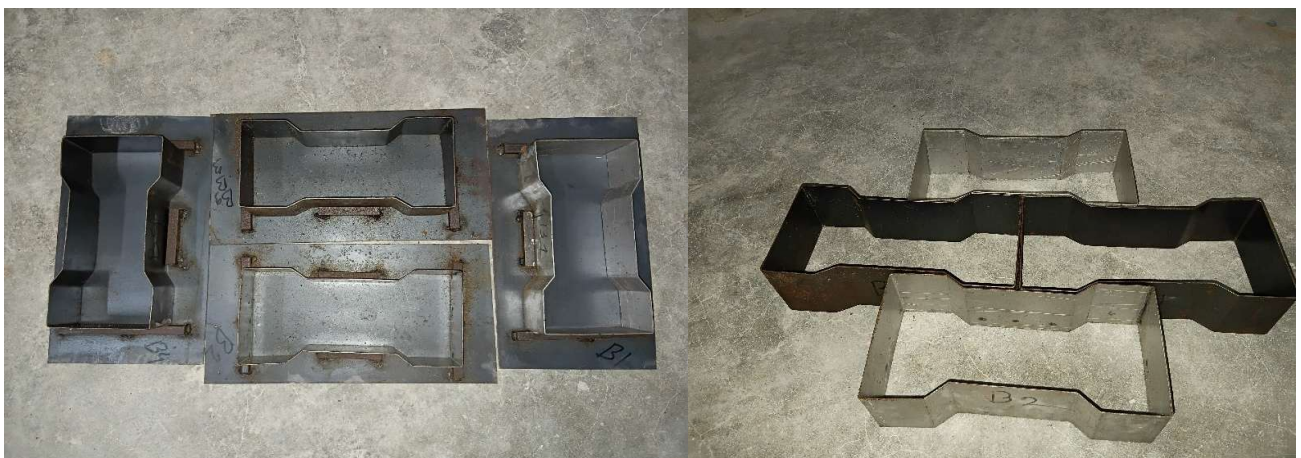
Figure 4: Brick Forma, made of Mild Steel Sheet
