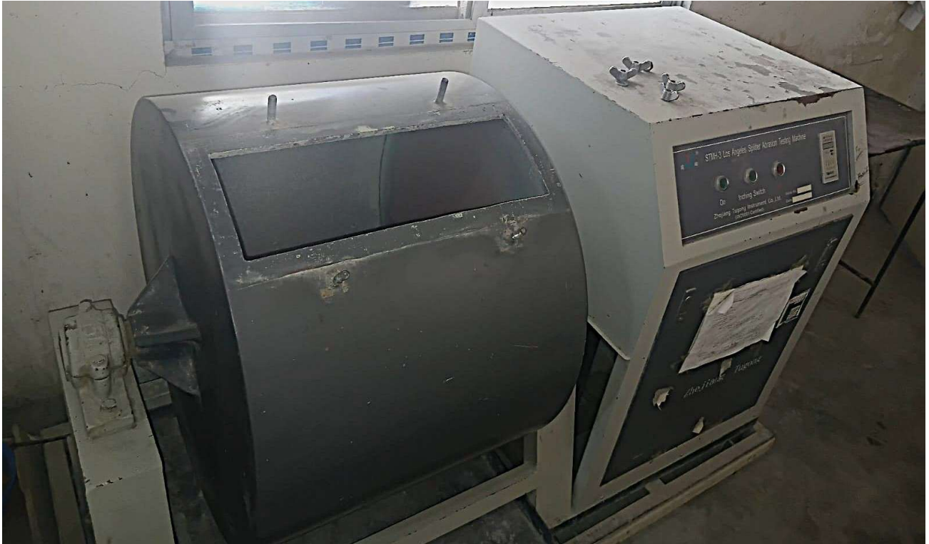
Figure 19: Los Angeles (LA) Abrasion Machine.
