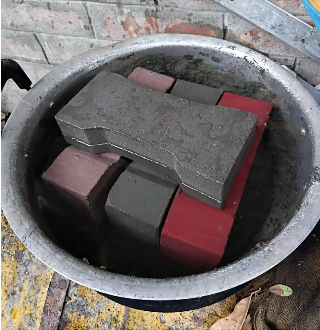
Figure 17: Curing of Brick
