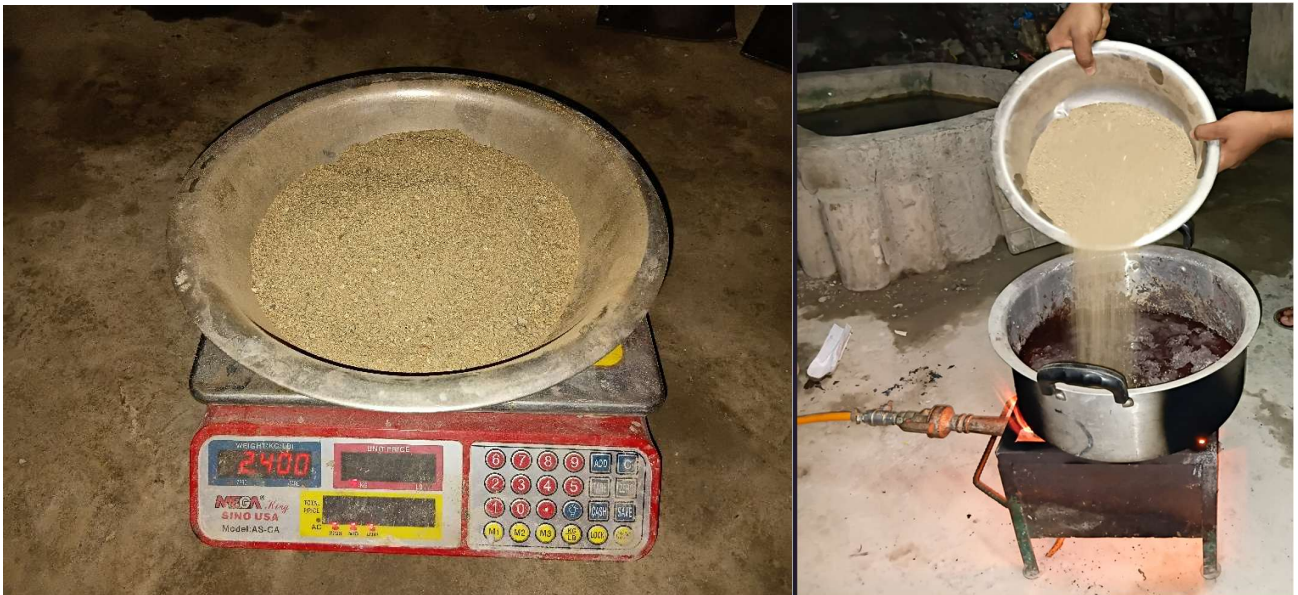
Figure 13: Adding Sand to melted Plastic
