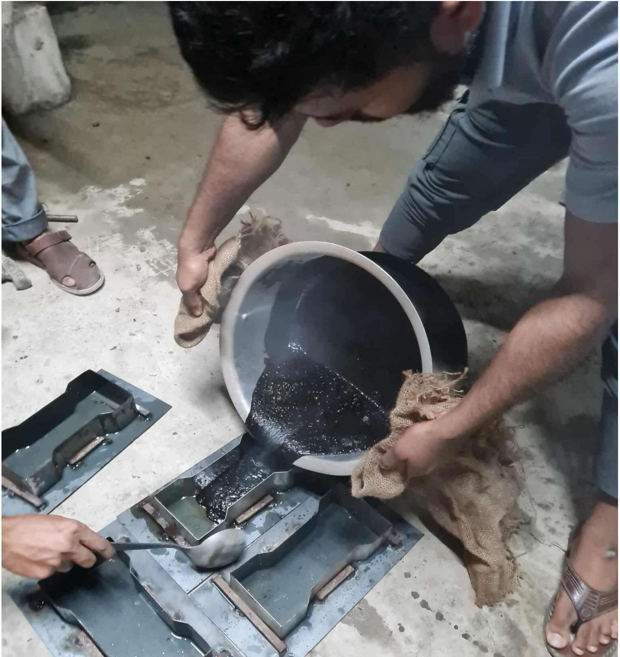
Figure 14: The mixer is pouring into the mold
