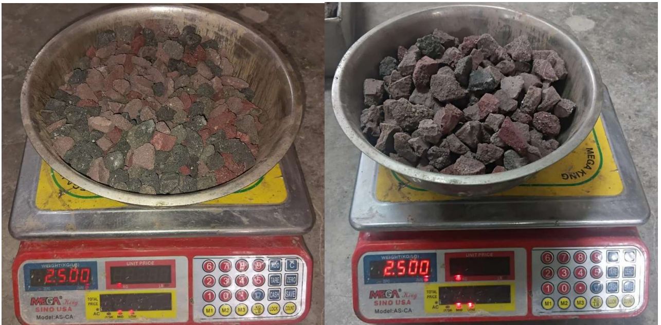
Figure 21: Weighing the Khoa for the Abrasion test.
