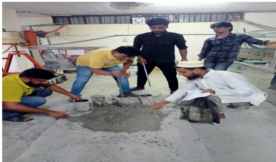
Figure: 3.11 Concrete Mixing And Molding
