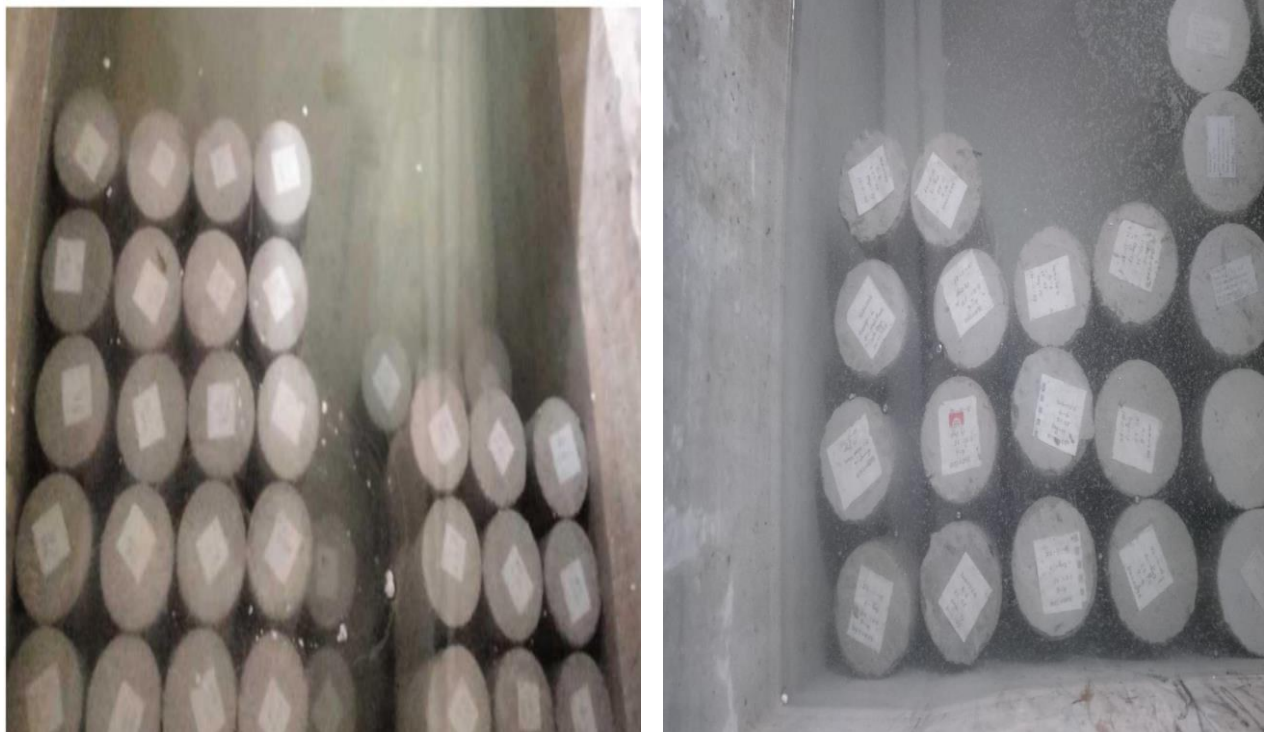
Figure: 3.13 Curing Process
