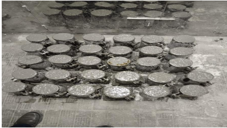
Figure: 3.12 Mold of Cylinder
