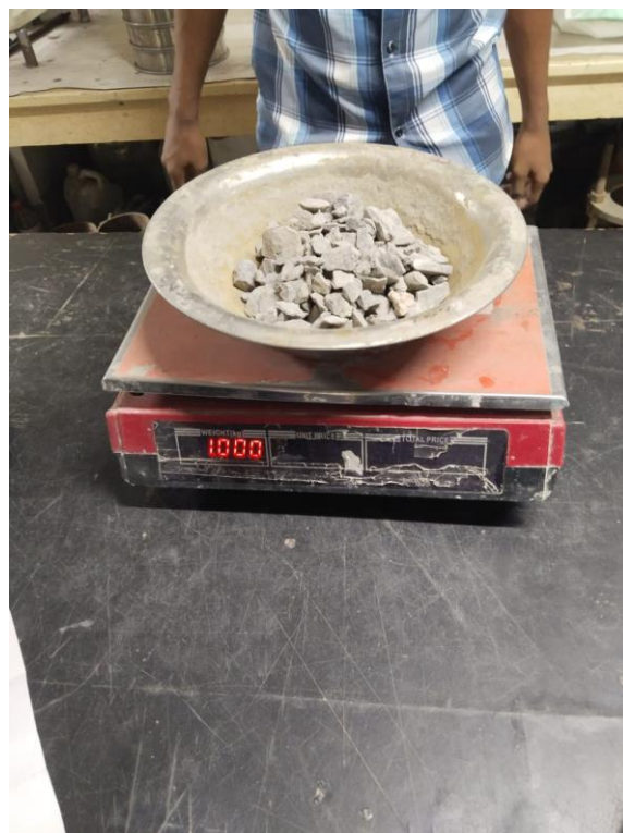
Figure :3.9 Sieve Analysis of Stone
