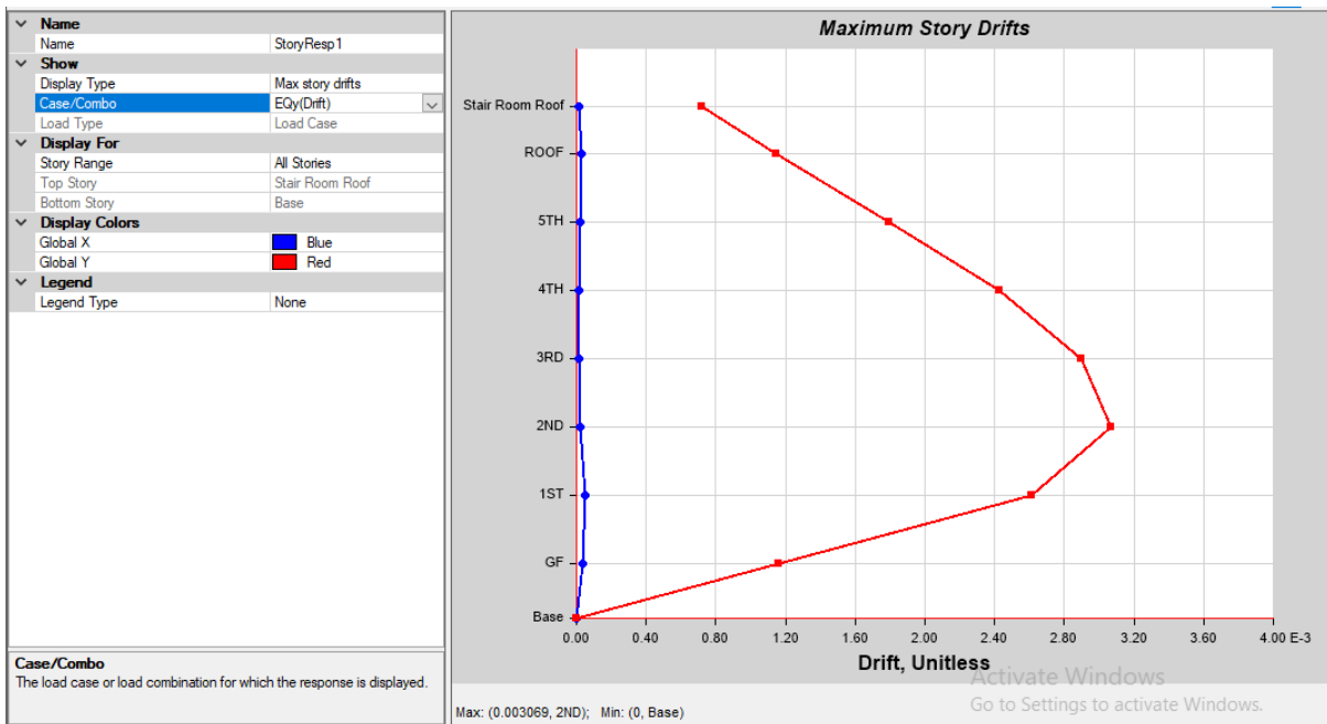
Figure 4.10: Maximum Story Drift With Retrofitting (EQy)
