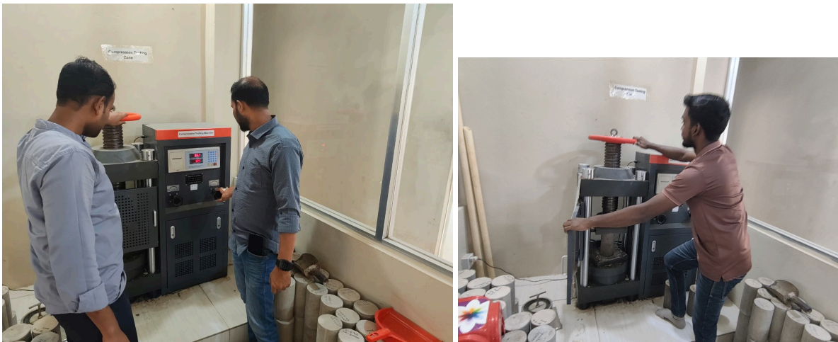
Figure 3.8 (b) : Cylinder Crushing
