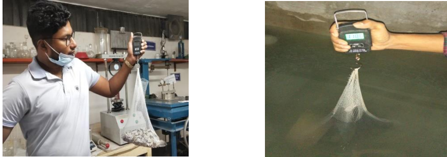
Figure 4.4: Specific gravity tests
