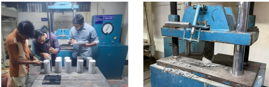
Figure 3.6: Compressive Strength Test of concrete cylinder
