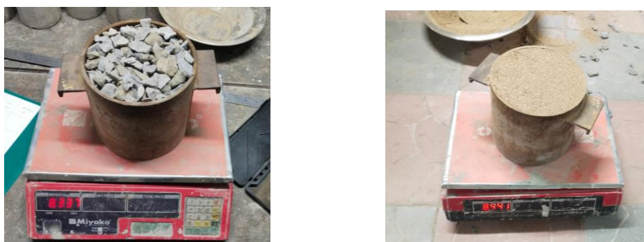
Figure 4.5: Unit weight of aggregate tests
