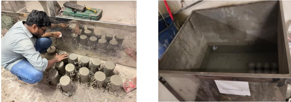
Figure 3.5: Cylinder leveling and curing
