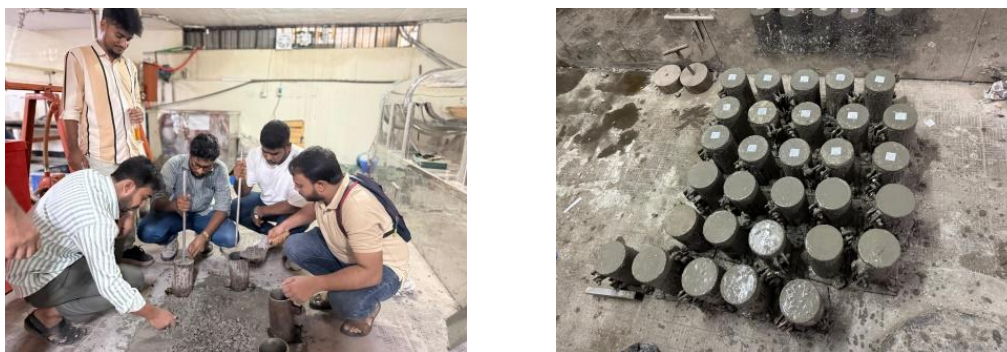
Figure 3.4: Materials pouring in the mold, temping and Cylinder making
