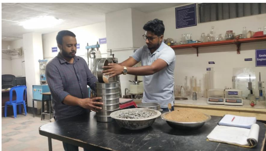
Figure 4.1: Sieve Analysis test
