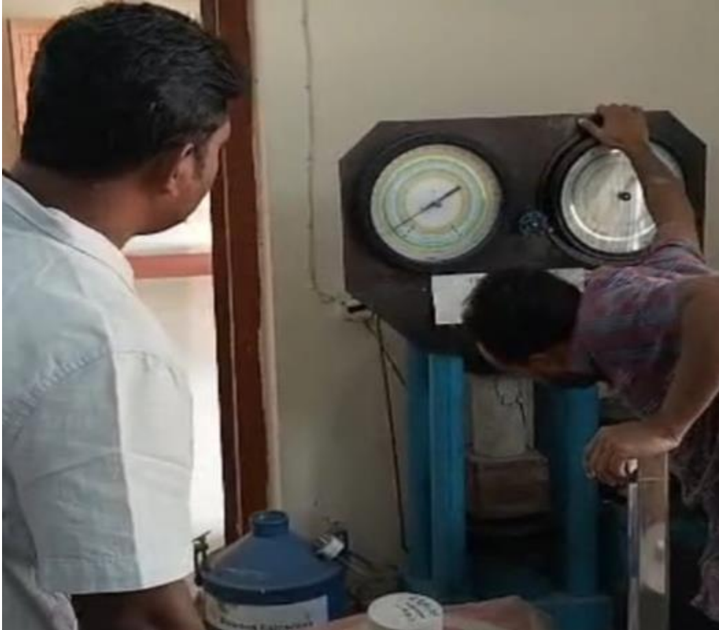
Figure: Concrete Cylinder Crushing by UTM
