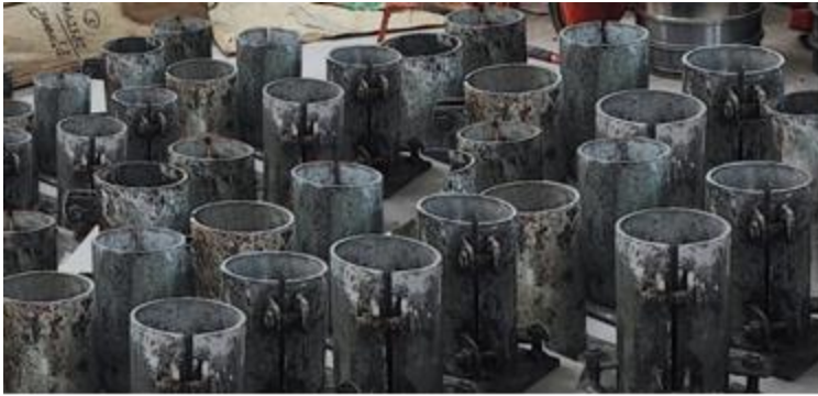
Fig: Preparation of Cylinder (150mm x 300mm)
