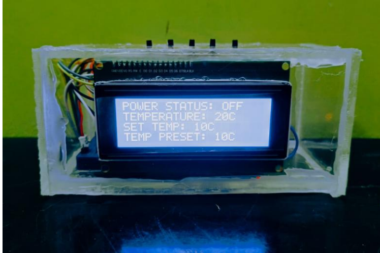
Figure 5.3: Control Box of the Smart Refrigerator
