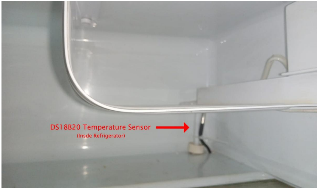
Figure 3.6: Temperature Sensor (Inside Cooling chamber)
