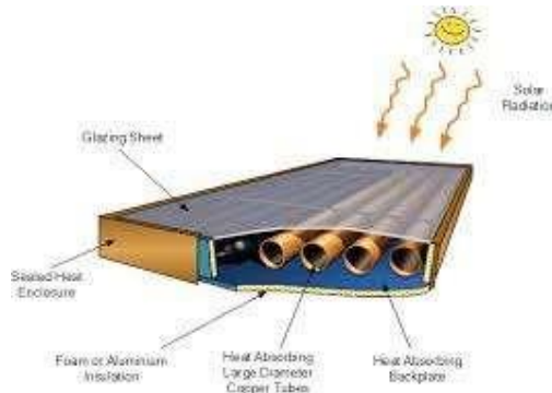
Figure-2.8: Integral Collector Storage System [10]
