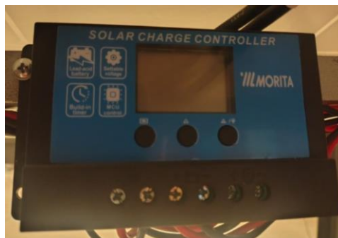
Figure-3.3: Solar Charge Controller
