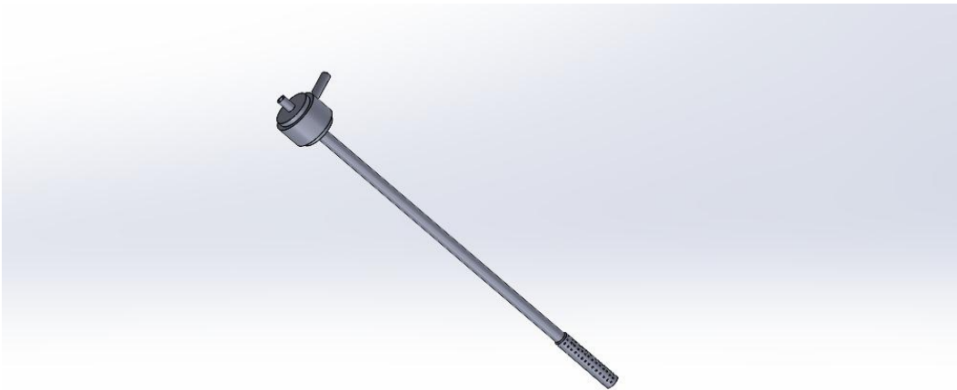
Figure 1: Vortex Tube components designed in SolidWorks
