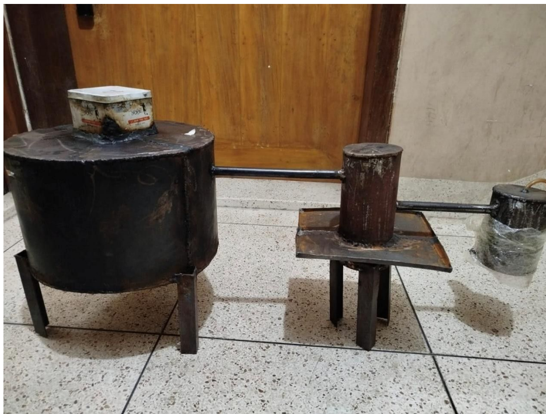
Fig-3.2.1: Main setup for Plastic Pyrolysis System
