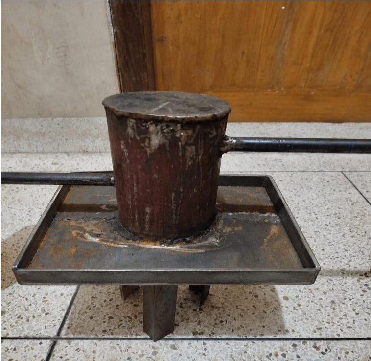
Fig-3.5.4: Condenser (Water Tray)
