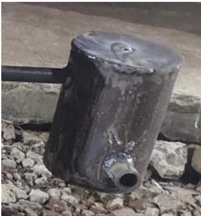
Fig-3.5.6: Fuel Collection Tank
