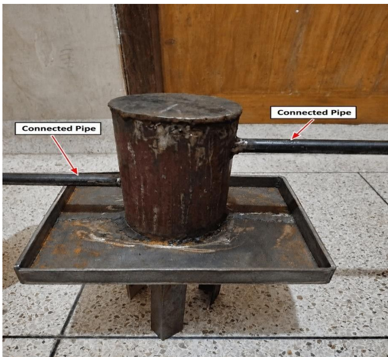
Fig-3.5.5: Connecting Pipe
