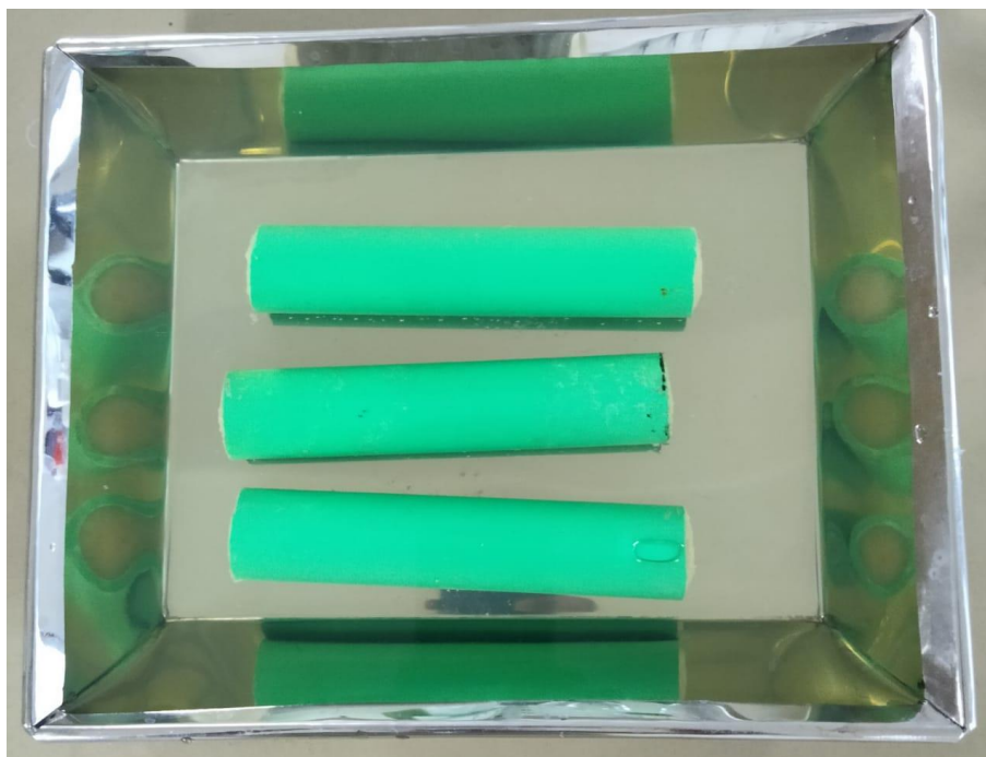
Figure 6: Crosslinking of PEM by glutaraldehyde (2.5% v/v)
