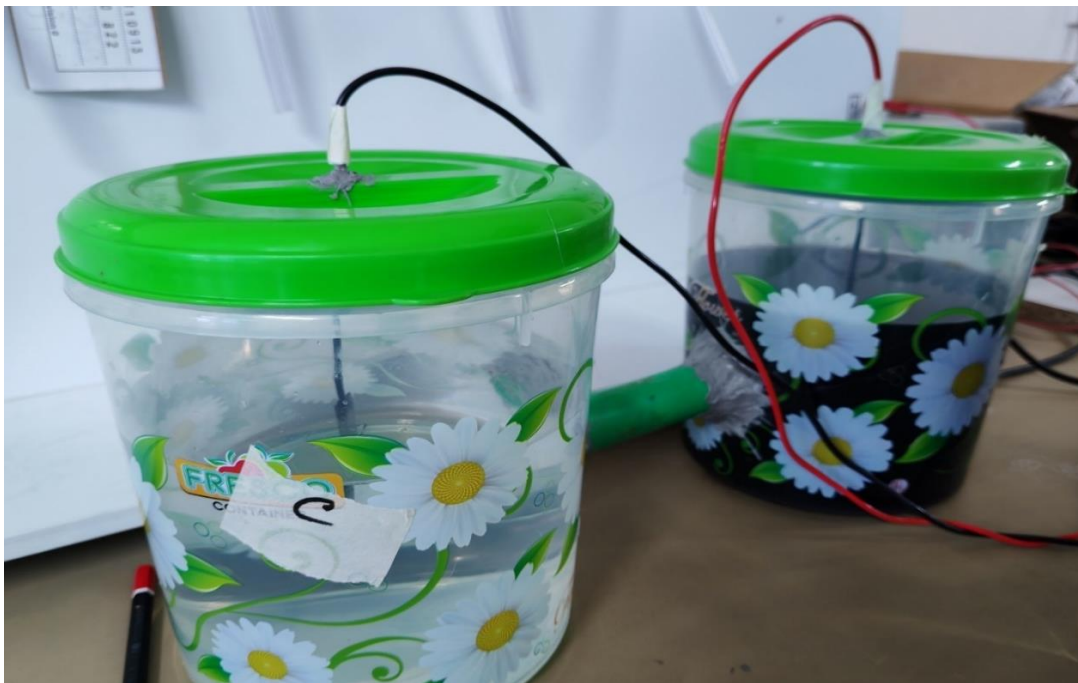
Figure 3: Two chambers of MFCs for a conventional membrane
