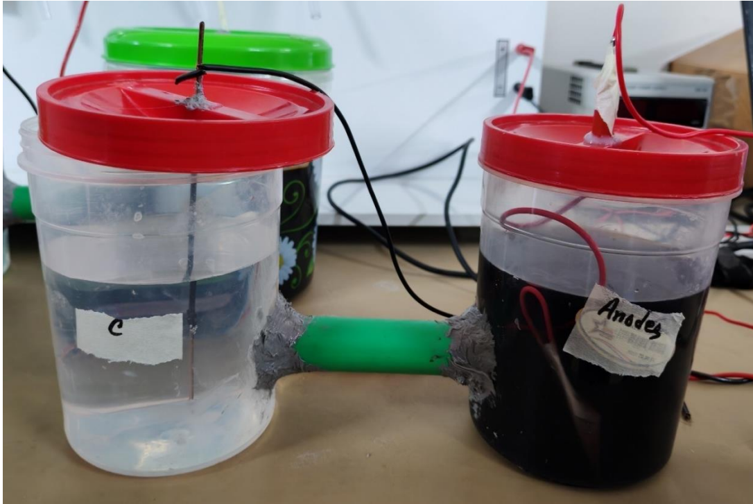
Figure 2: Two-chamber MFCs for composite membrane.
