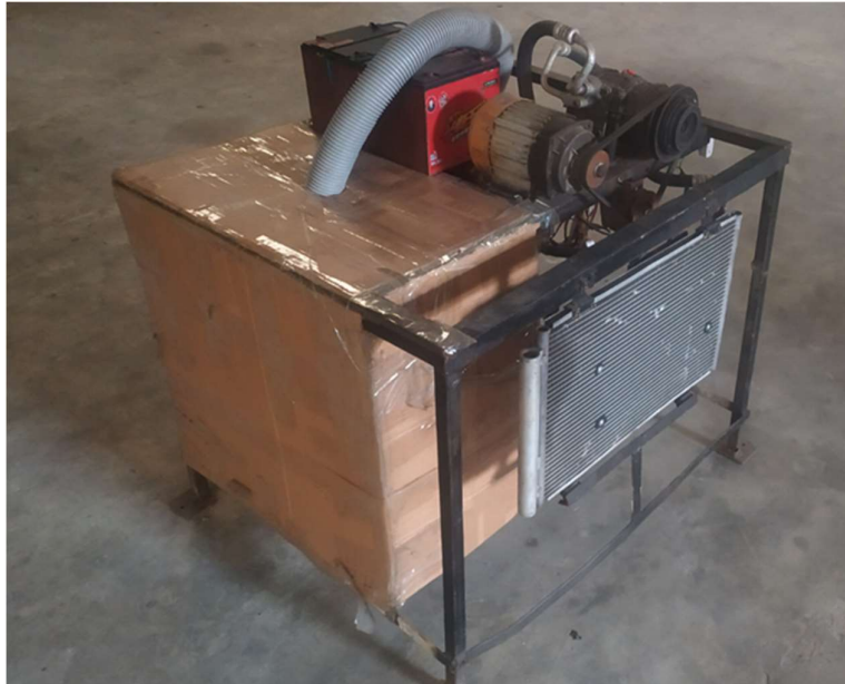
Figure 12: Backup Air-conditioning system by Battery Energy.
