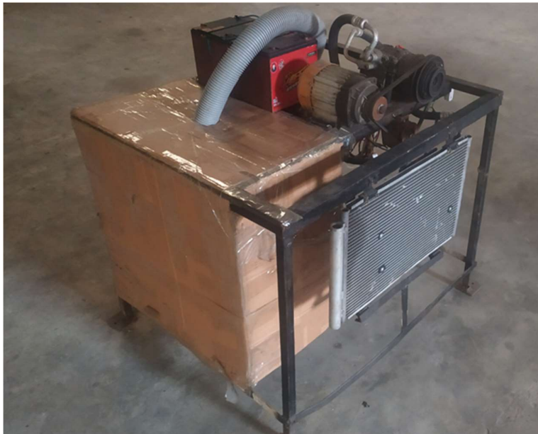
Figure 17: Assembling of all the components of backup Air-conditioning system in Air-conditioned vehicle.
