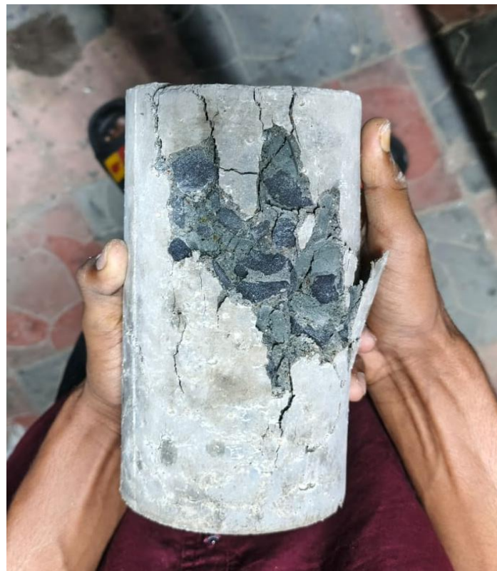
Figure 3.17: Compressive Fracture of Cylinder after 28 Days
