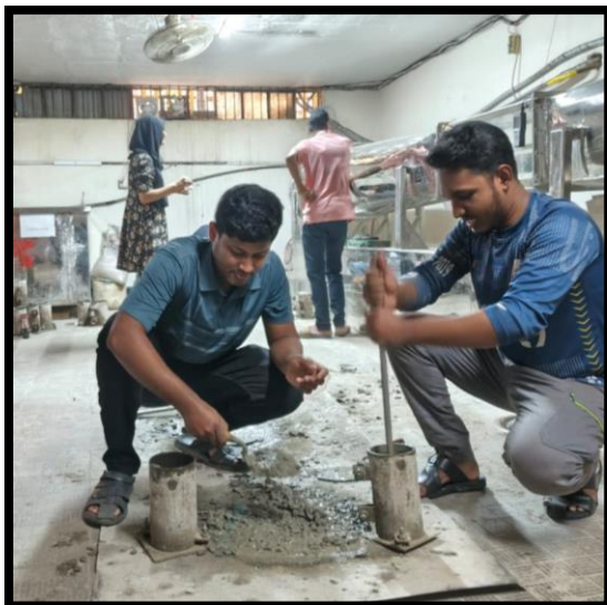
Figure 3.7: Mold Filling with Concrete and Tamping
