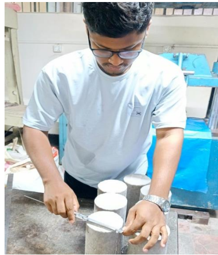
Figure 3.14: Measuring cylinder's Dia by Vernier Caliper
