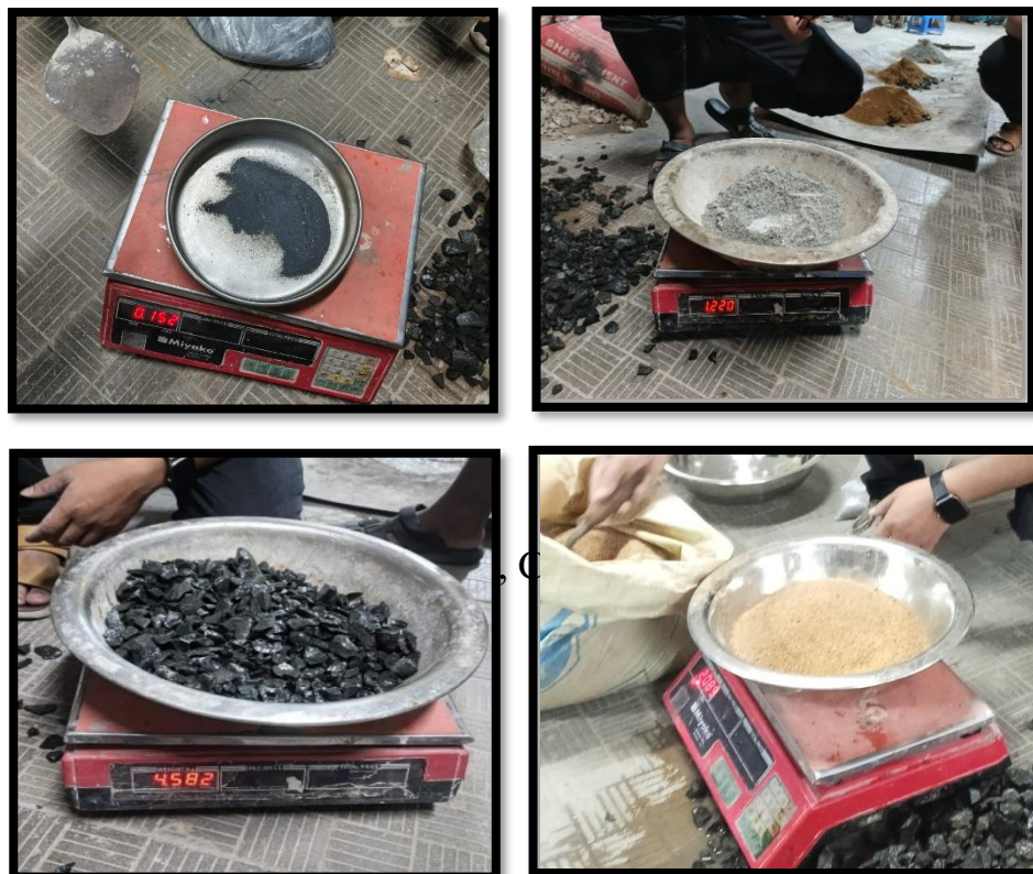
Figure 3.5: Measurement of Slag, Cement, Stone & Sand
