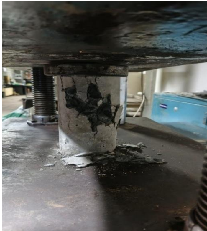
Figure 3.16: UTM Load Application
