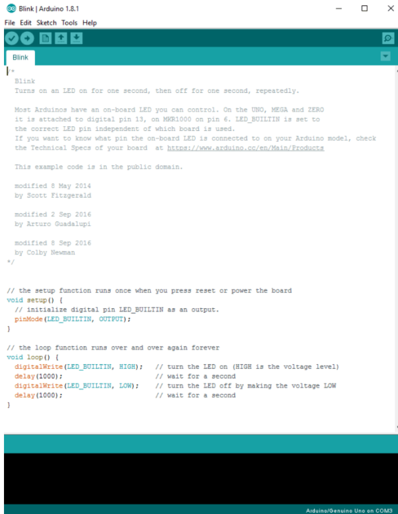
Figure 3-15: Basic program of LED Blinking
