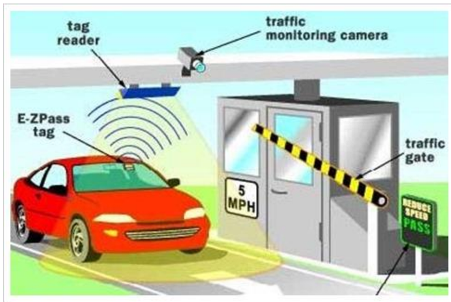
Figure 2.2: A toll collection system utilizing RFID
