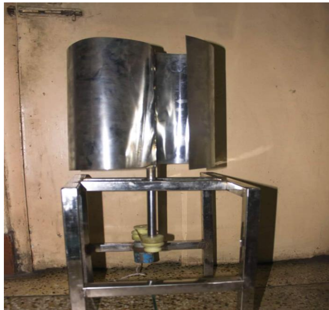
Fig 3.1: Savonius wind turbine with 4 blades
