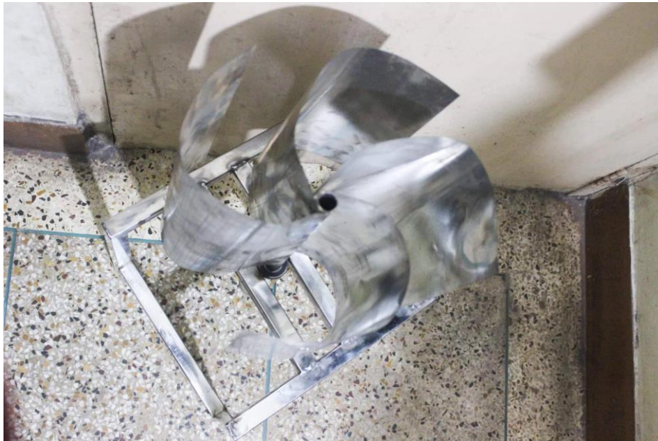
Fig 3.4: Small 4 blade Savonius wind turbine
