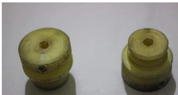
Fig 3.7: Shaft and generator motor pulley
