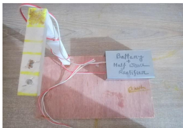
Fig 4.6: Energy storage & usage with LED
