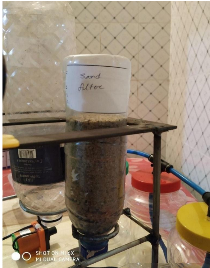
Fig: 4.7 Sand Filter
