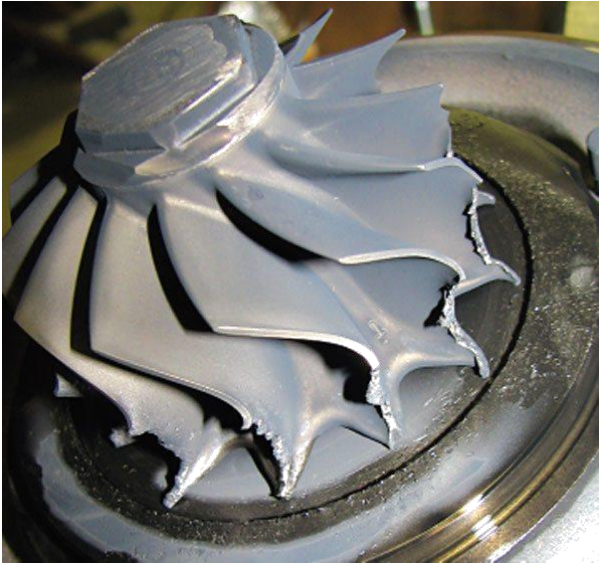
Fig. Faillure compressor
