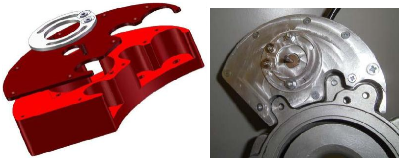
Fig. 5. The stepper motor housing assembly. In the left an exploded view of the 3D model and, at right, the referred part already fitted in the turbocharger.
