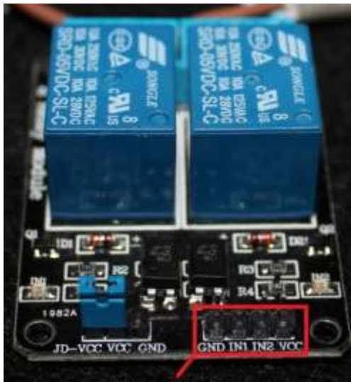
Figure 2.15: Main Voltage Connection
