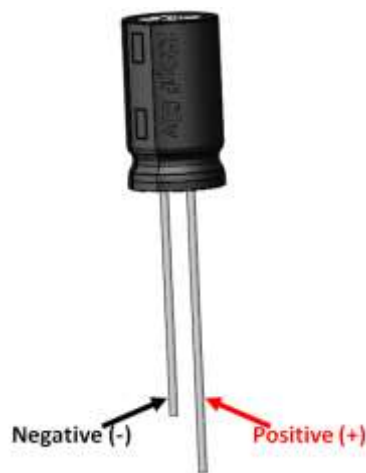
Figure 2.17: Capacitor Pin Out
