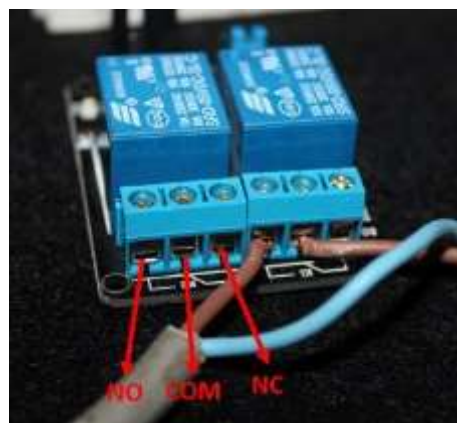
Figure. 3.16: Mains voltage connections.
