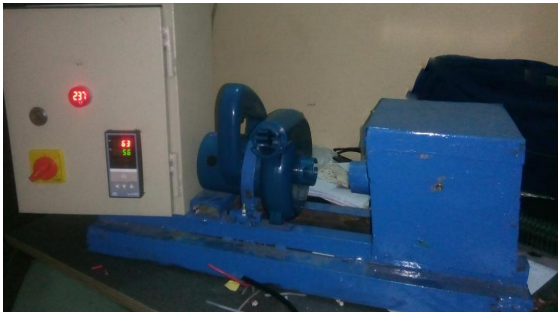
Figure 3.1: Automatically Controlled Industrial Air Heat Blower and Chamber System.
