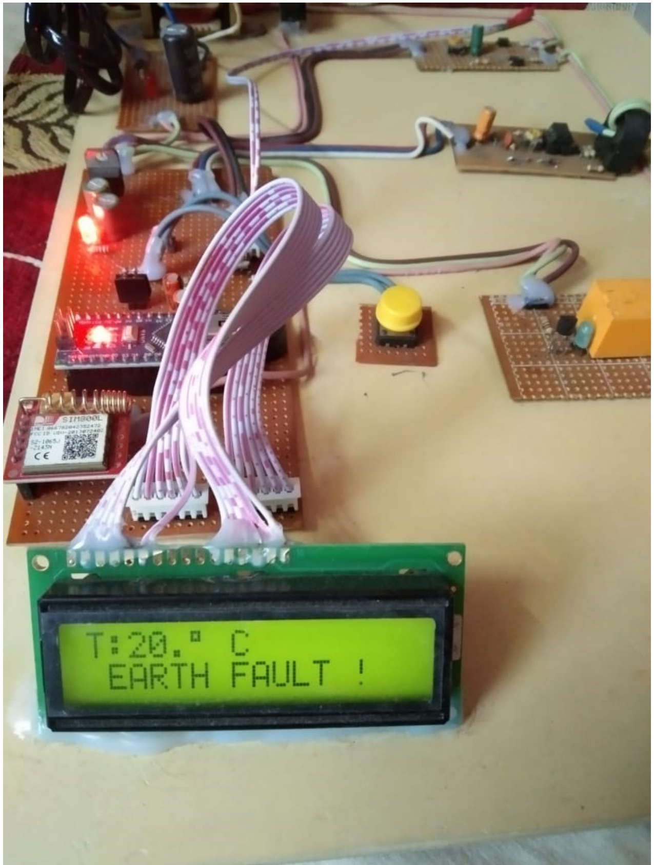
Figure 5. 1 Earth fault result
