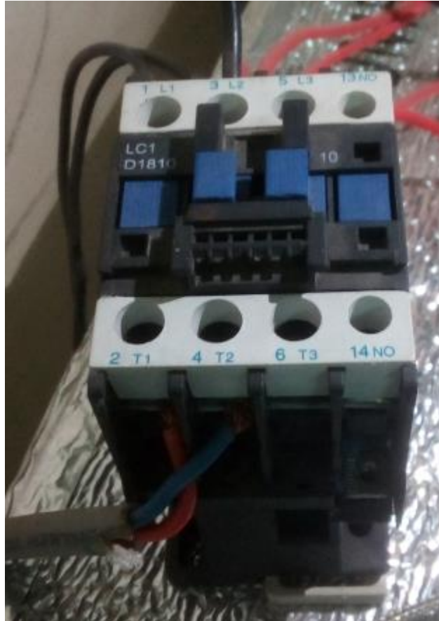
3.7 Figure: Electric contractor
