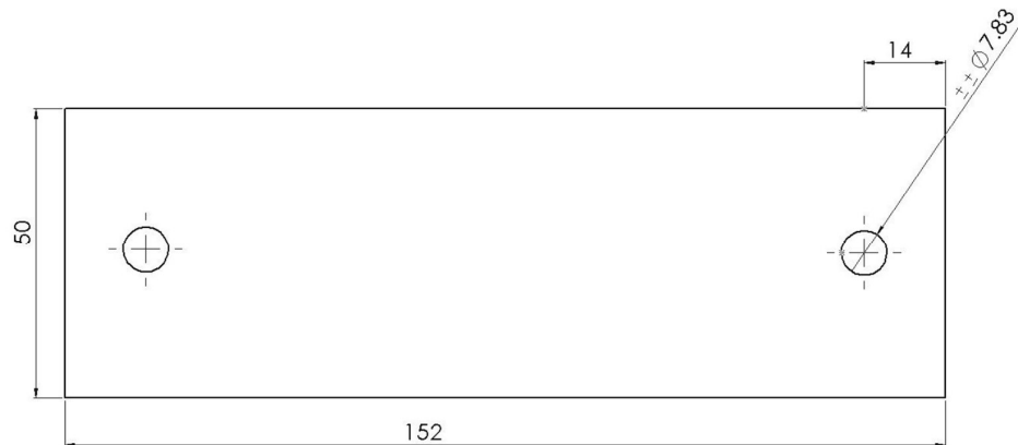
Figure 4.1.1.1.1a: Schematic view of Base V.01
