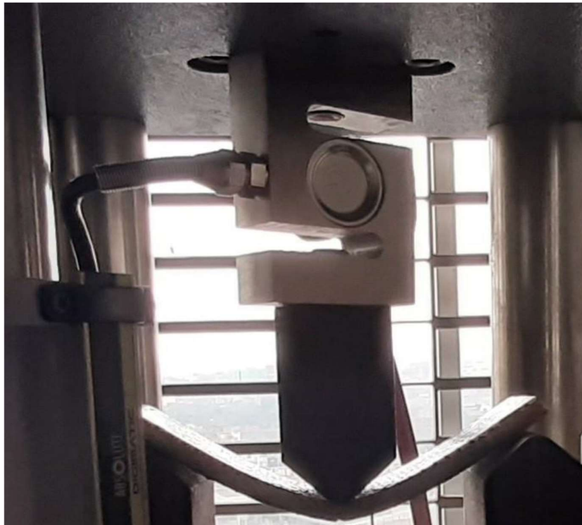
Figure 4.1.1.3.3: Indenter with sensor attached
