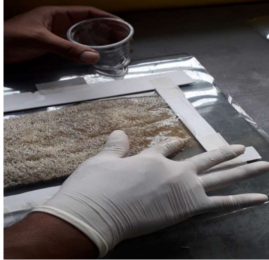
Figure 3.1e: Mixture is being poured on to the surface of the fiber and Polyester
