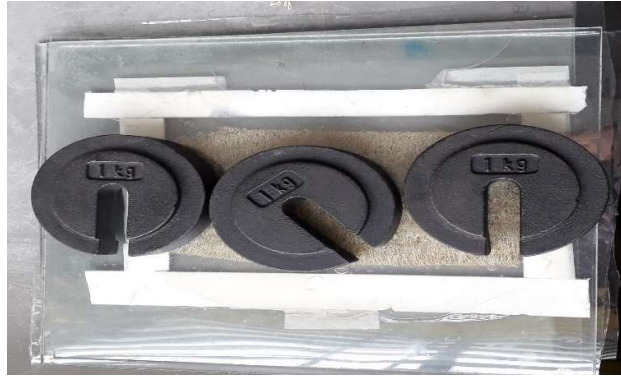
Figure 3.1g: A regular notched 1+1+1= 3 kg weight placed on top of the fabricated composite material
