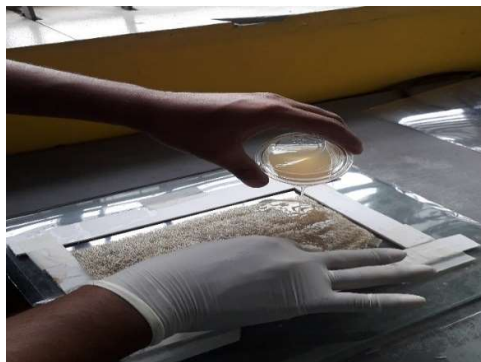
Figure 3.1d: Mixture is being poured on to the surface of the fiber and a cylindrical roller is used for the spreading
