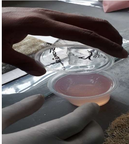
Figure 3.1c: Mixing of Polyester and hardener
