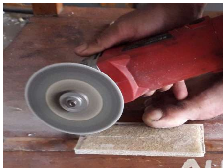
Figure3.1j: Manual grinding operation
