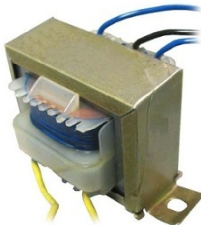
Figure 2.14: 220v to 12V step down transformer.
