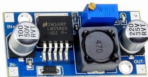
Fig 2.19: DC-DC Buck Converter
