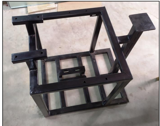
Figure: 3.5.1.1. Supporting Frame of Hammering Machine
