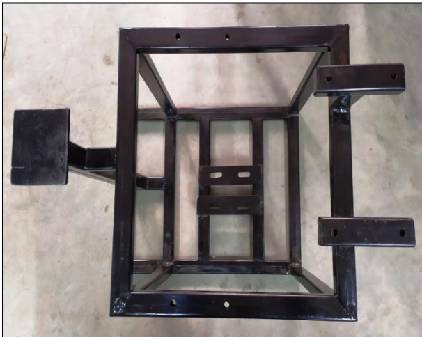
Figure: 3.5.1.1. Supporting Frame of Hammering Machine
